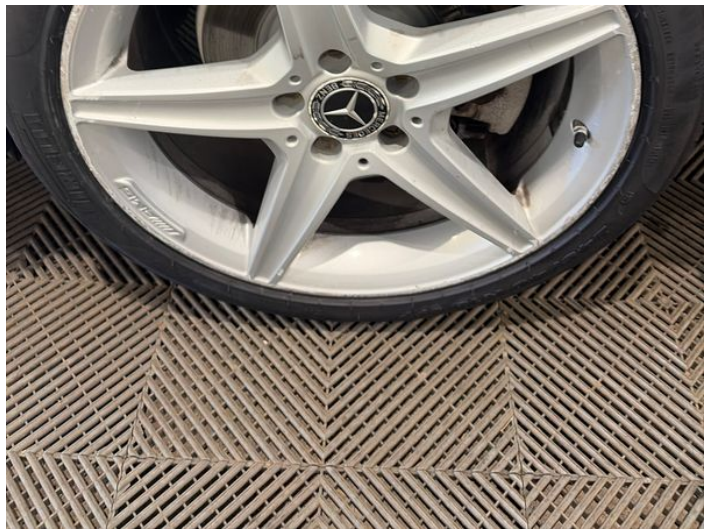
12: Wheel nsr Scratched Over 50mm
