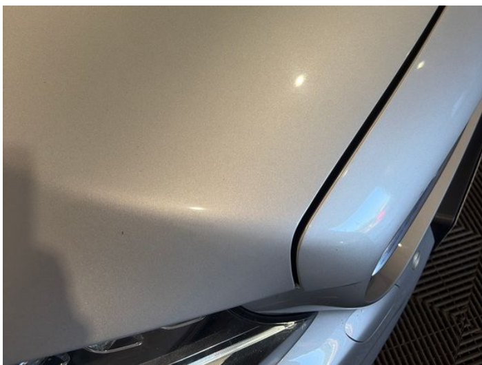
5: Bonnet Poor Previous Repair Poor Paint
