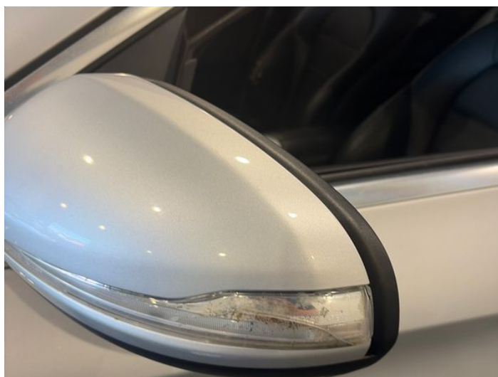
8: Flasher Side Repeater ns Broken Replace
