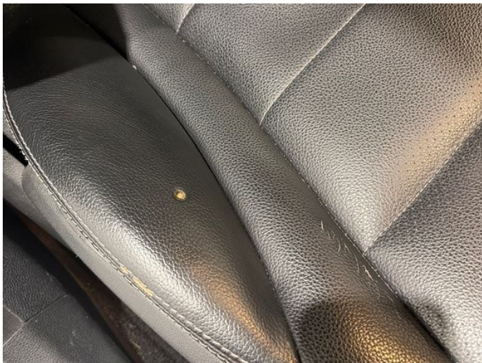
3: Seat Back Cover osf Burn Over 3mm
