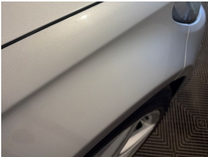
21: Wing osf Poor Previous Repair Poor Paint
