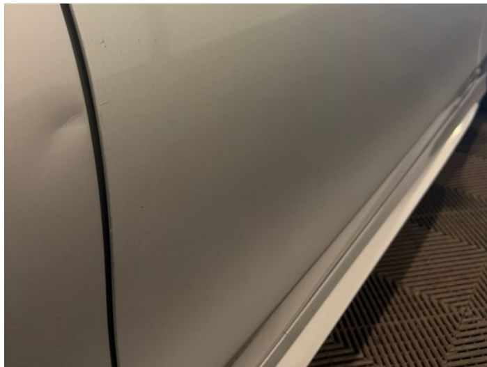
18: Door osf Dented With Paint Damage
