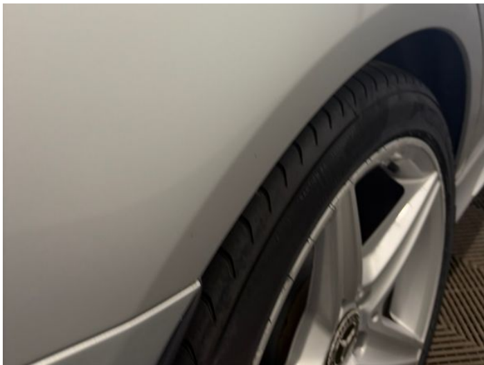
15: Qtr Panel osr Scratched Over 25mm Thru Paint
