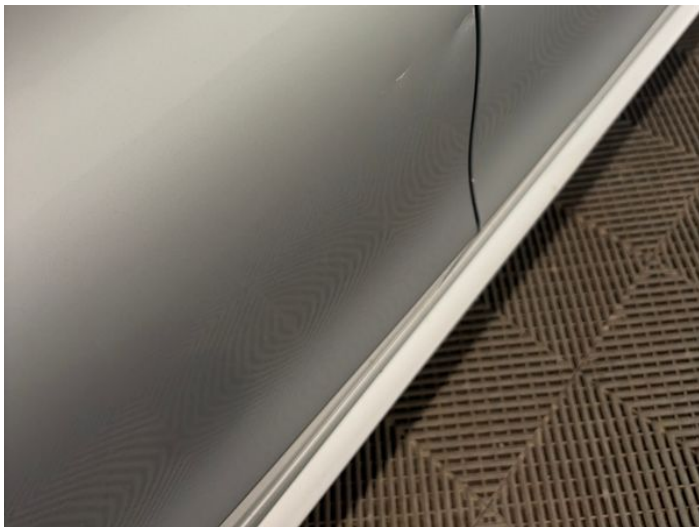
17: Door osr Dented With Paint Damage
