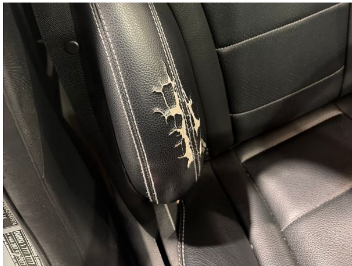
4: Seat Back Cover osf Torn Over 3mm
