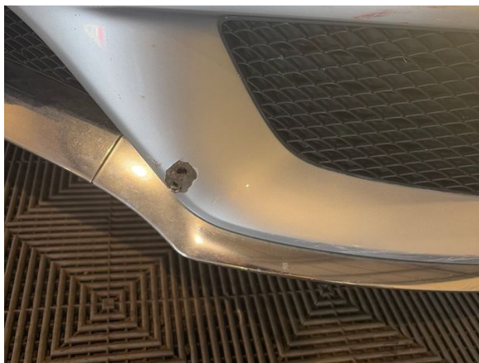
6: Bumper Front Hole Over 25mm
