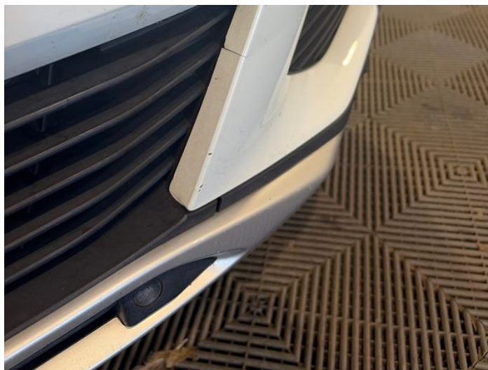
2: Bumper Front Cracked UpTo 25mm
