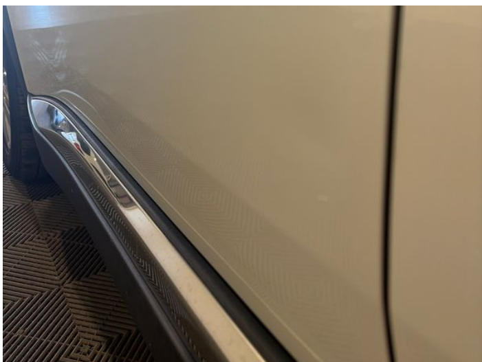
5: Door nsf Dented Between 10mm + 30mm
