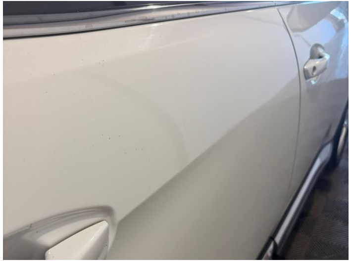
10: Door osr Poor Previous Repair Rippled UpTo 30%
