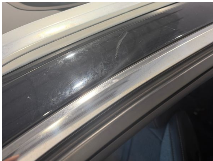
4: A Post ns Scratched Over 25mm Thru Paint
