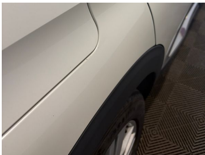
8: Qtr Panel osr Dented Between 10mm + 30mm
