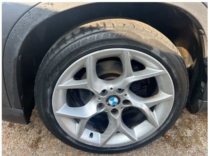
8: Wheel nsf Scratched Over 50mm
