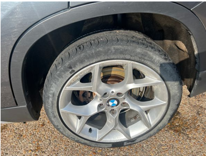
5: Wheel nsr Corroded Light
