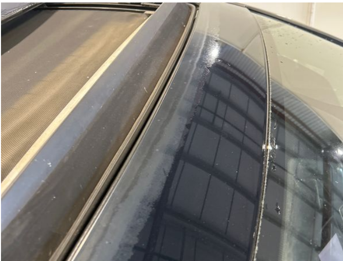
23: Roof Scratched Over 25mm Thru Paint
