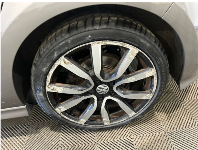
13: Wheel nsr Corroded Light
