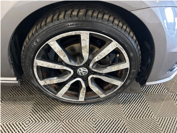
3: Wheel osf Corroded Light
