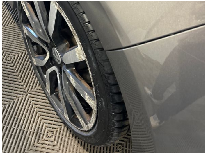
12: Qtr Panel nsr Dented Over 30mm
