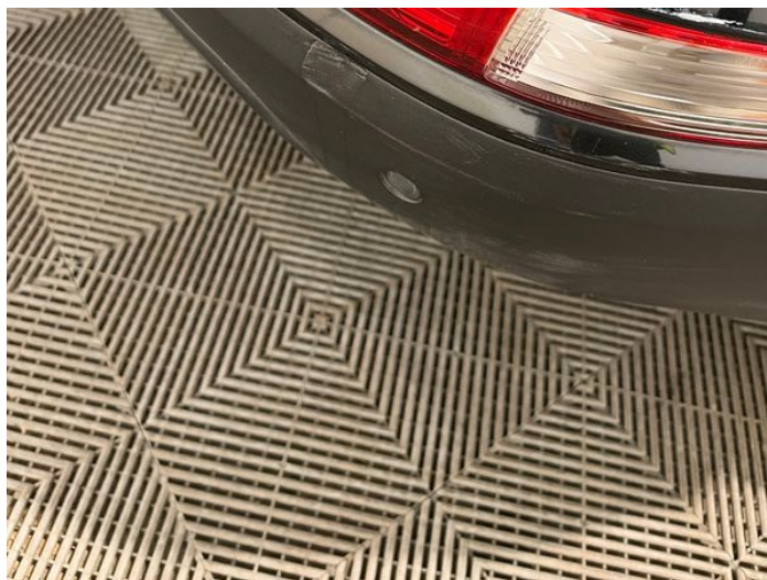
22: Bumper Rear Moulding Scuffed (Unpainted) Over 100mm
