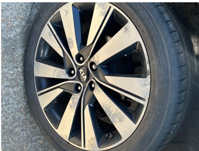
11: Wheel nsr Corroded Light
