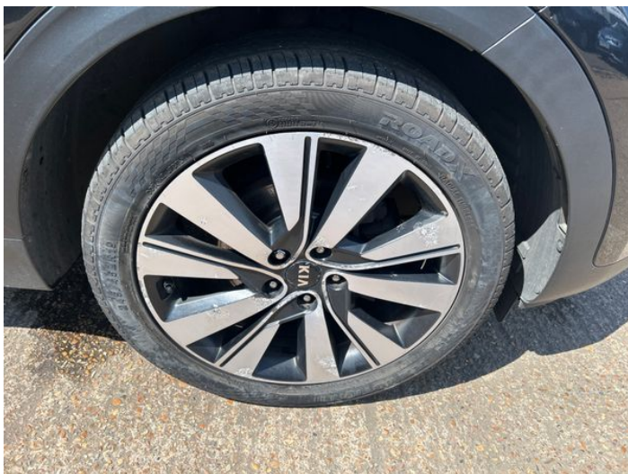
1: Wheel osf Corroded Light
