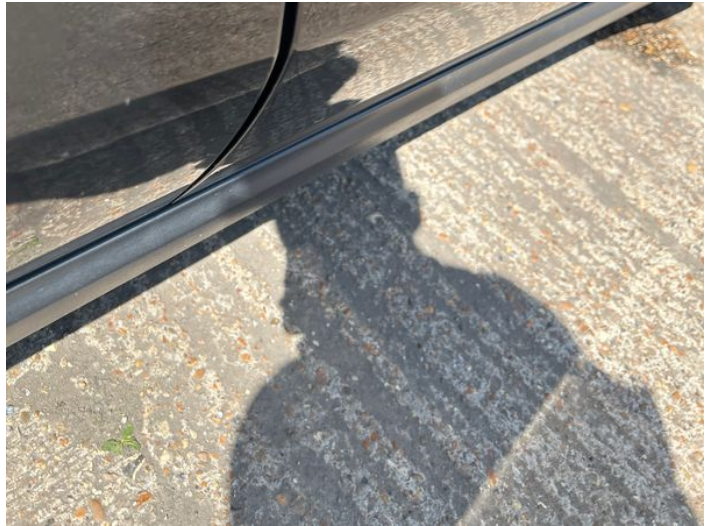
4: Door osf Chipped Edge Chip
