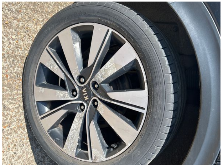
6: Wheel osr Corroded Light
