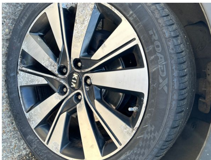
14: Wheel nsf Corroded Light
