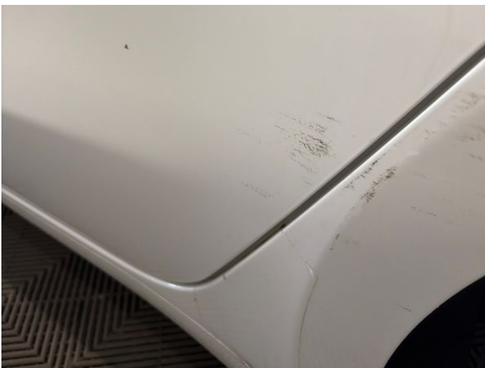
7: Door nsr Scratched Over 25mm Thru Paint
