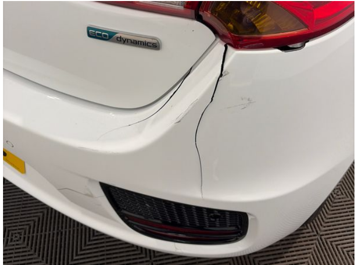
10: Bumper Rear Cracked Over 25mm
