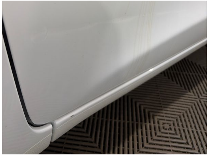
4: Door nsf Dented Over 30mm
