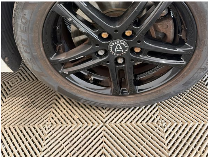
15: Wheel osf Scratched Over 50mm
