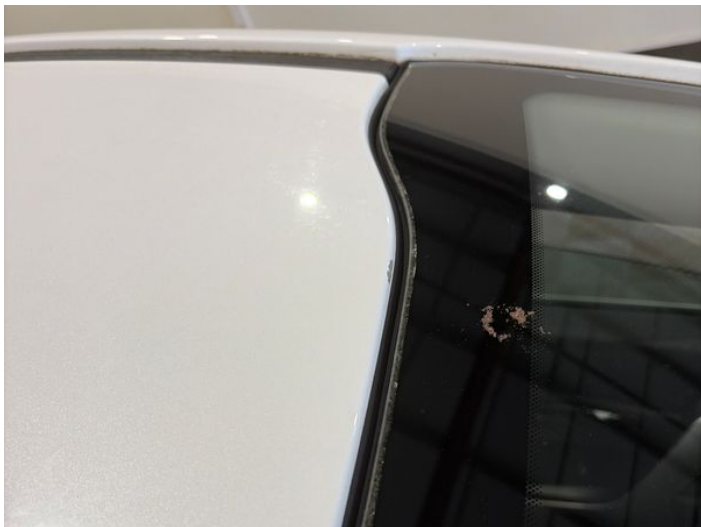
17: Roof Chipped Edge Chip
