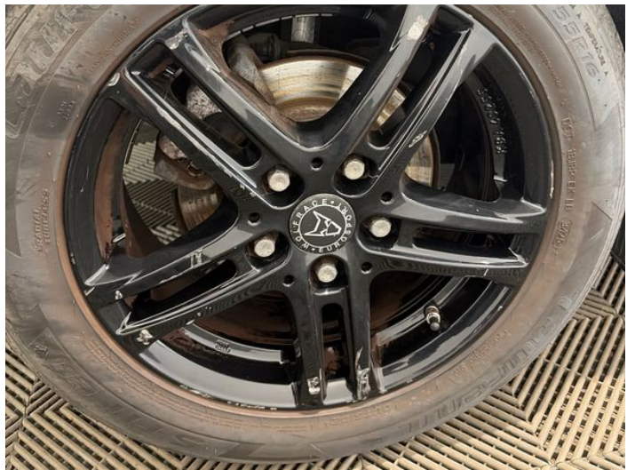
12: Wheel osr Scratched Over 50mm
