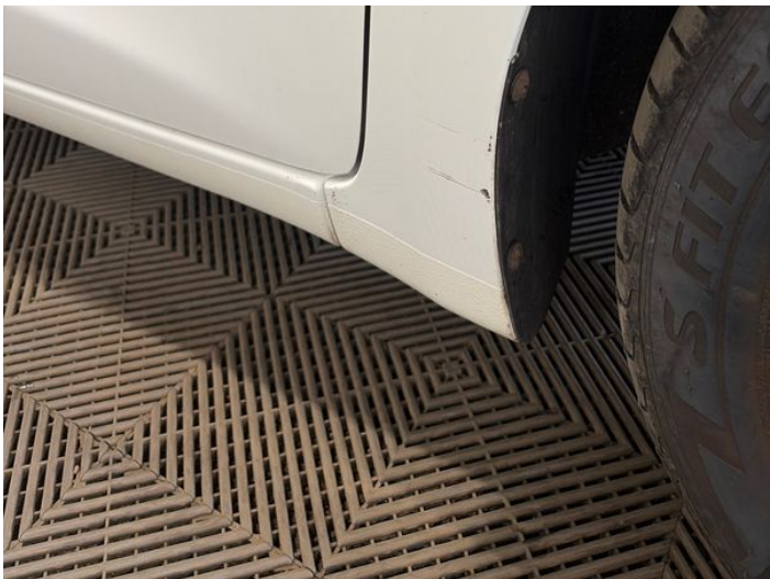
16: Wing osf Scratched Over 25mm Thru Paint
