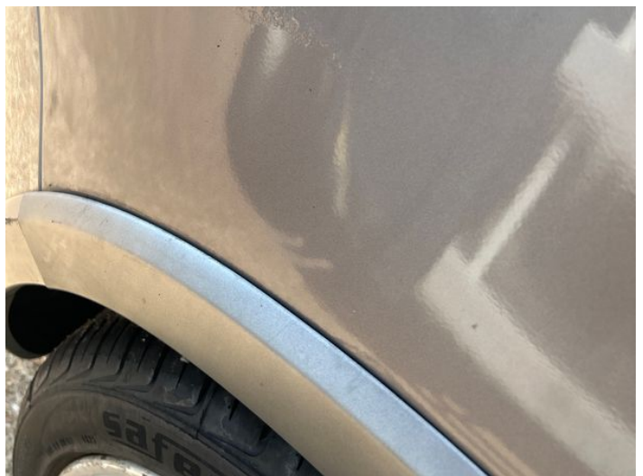
8: Qtr Panel osr Rusted Over 5mm
