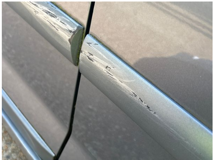
6: Door Moulding osf Scratched (Painted) Over 25mm Thru Paint
