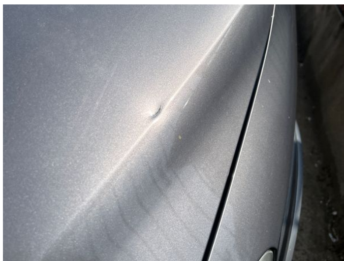
26: Bonnet Dented With Paint Damage
