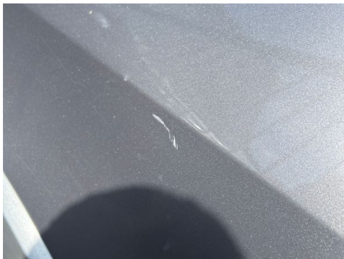
22: Wing nsf Scratched UpTo 25mm Thru Paint
