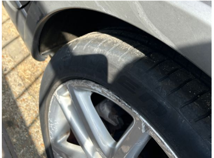
16: Qtr Panel Arch Extension ns Scratched (Painted) Over 25mm Thru Paint
