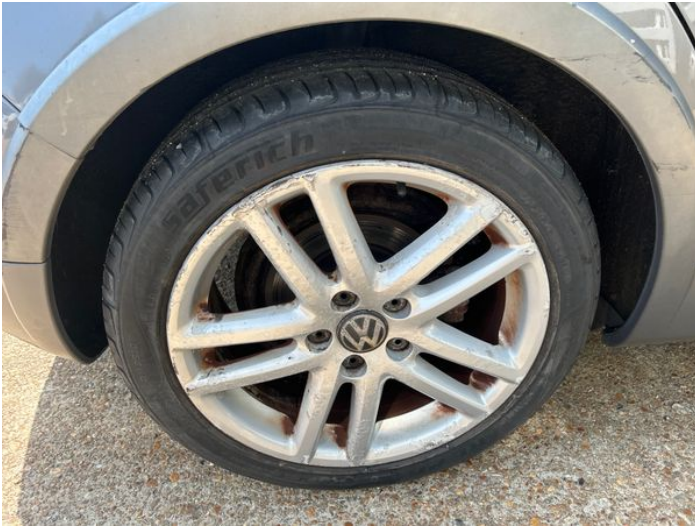
9: Wheel osr Corroded Light
