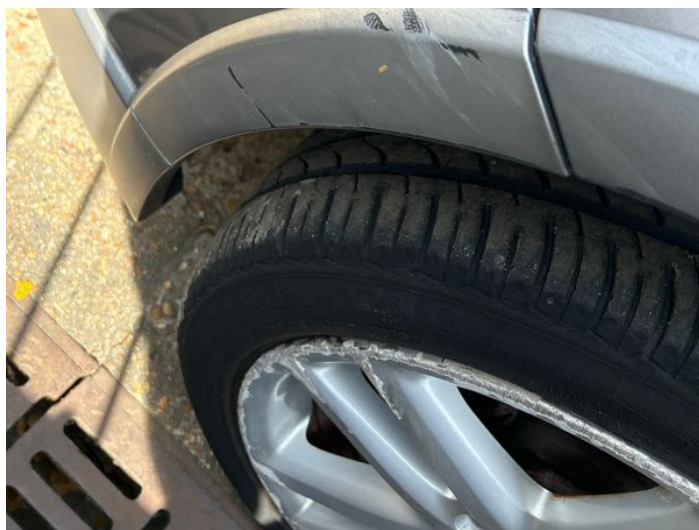
24: Bumper Front Moulding Scratched (Painted) Over 25mm Thru Paint
