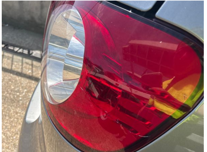
10: Lamp osr Broken Replace
