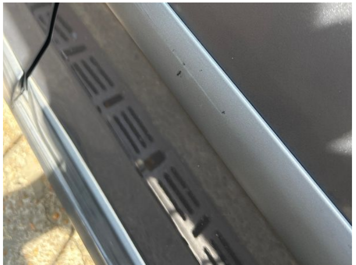
18: Door Moulding nsr Scratched (Painted) Over 25mm Thru Paint
