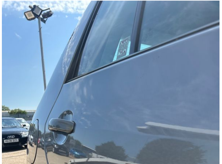
4: Door osr Dented Between 10mm + 30mm
