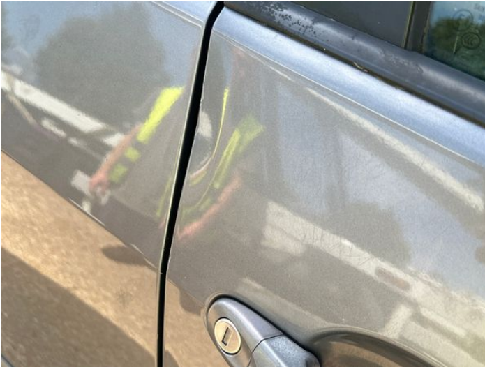
3: Door osf Dented Over 30mm
