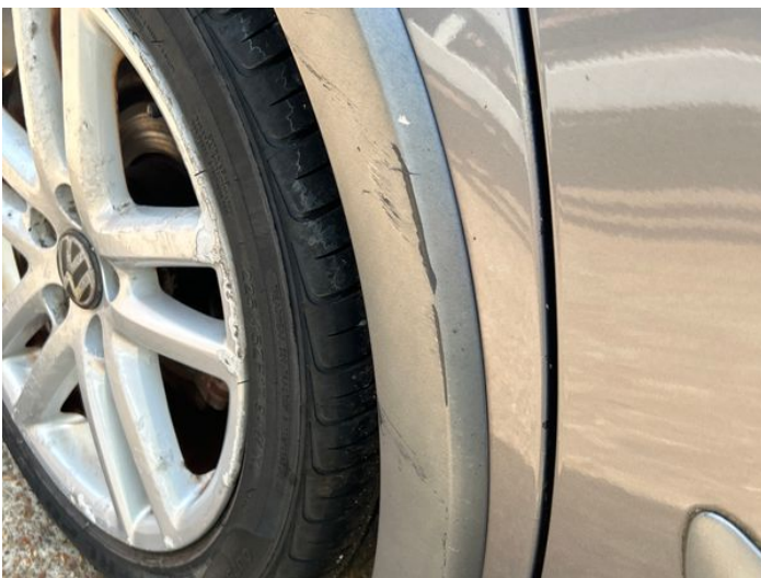
7: Qtr Panel Arch Extension os Scratched (Painted) Over 25mm Thru Paint
