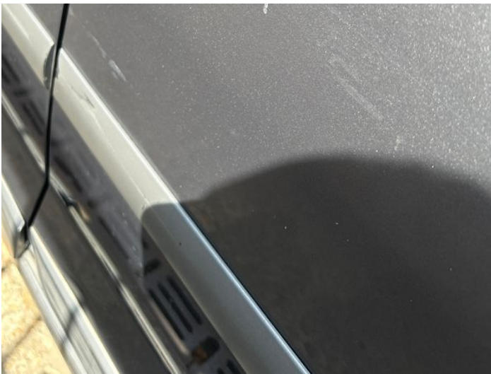
17: Door nsr Chipped 1 To 5
