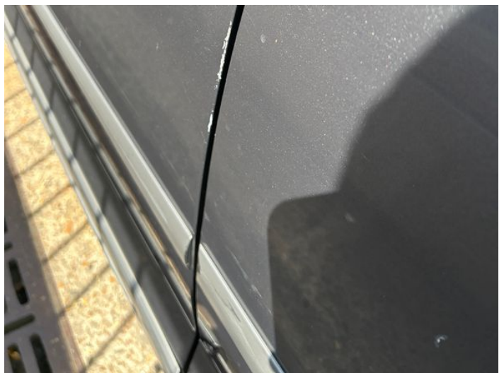
20: Door nsf Chipped Edge Chip
