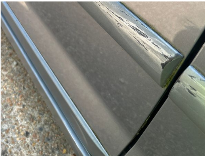
5: Door Moulding osr Scratched (Painted) Over 25mm Thru Paint
