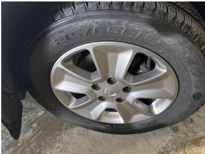
9: Wheel osf Scratched Up To 50mm
