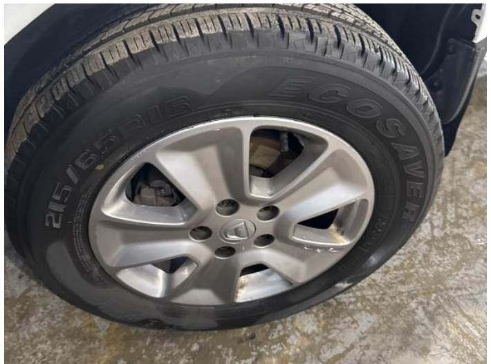
12: Wheel nsf Scratched Up To 50mm
