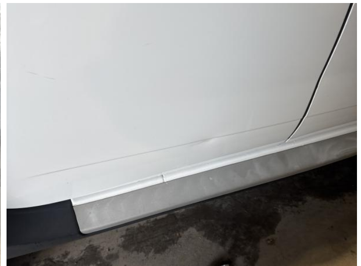
6: Door osr Dented Over 30mm
