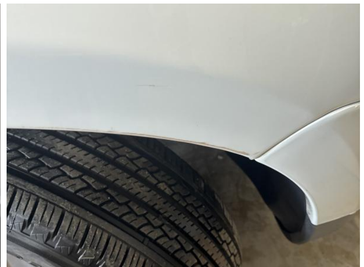
8: Wing osf Scratched UpTo 25mm Thru Paint
