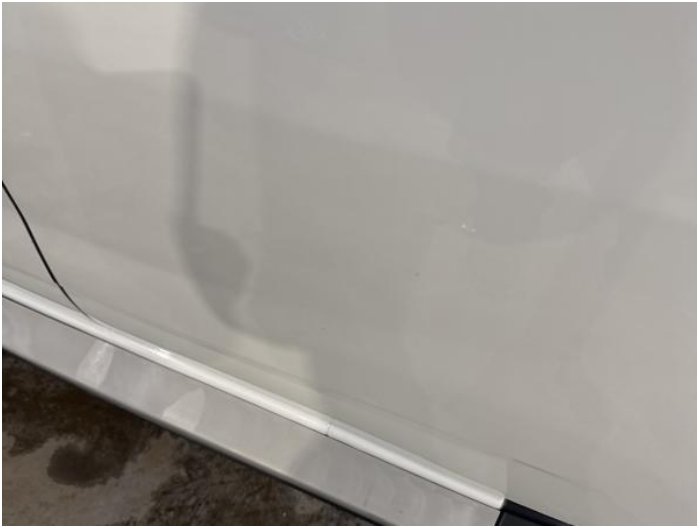
15: Door nsr Dented Between 10mm + 30mm
