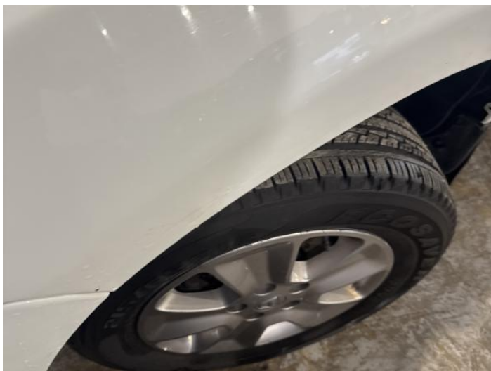
13: Wing nsf Scratched Over 25mm Thru Paint
