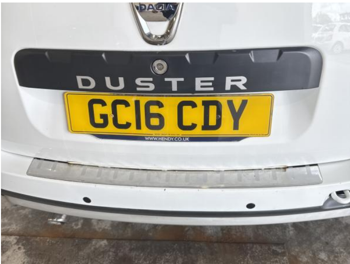
1: Bumper Rear Scratched 25 to 100mm Thru Paint
