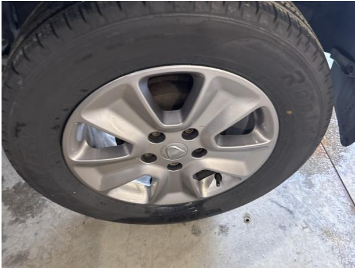
16: Wheel nsr Scratched Up To 50mm
