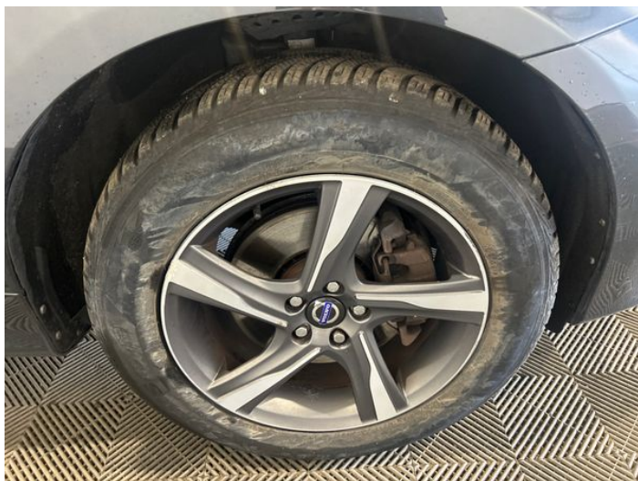
1: Wheel osf Corroded Light
