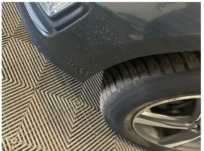
14: Bumper Front Scratched Over 100mm Thru Paint
