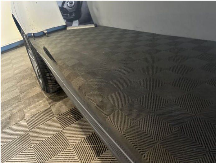
3: Door osf Dented Between 10mm + 30mm
