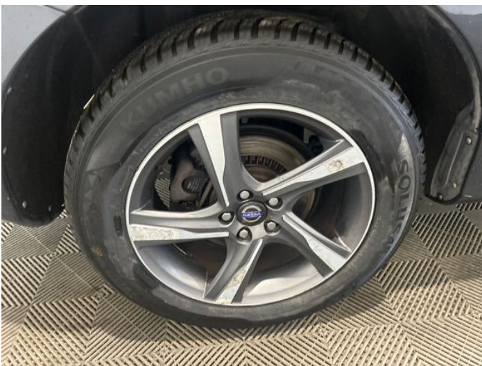
7: Wheel osr Corroded Light
