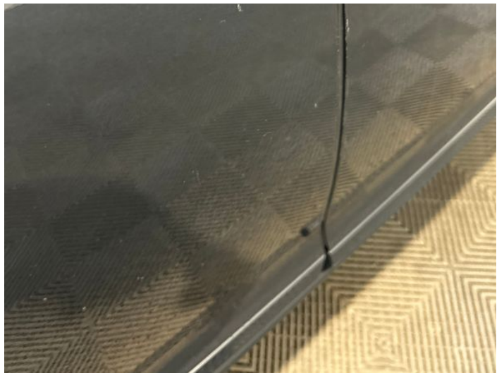
6: Door osr Scratched UpTo 25mm Thru Paint
