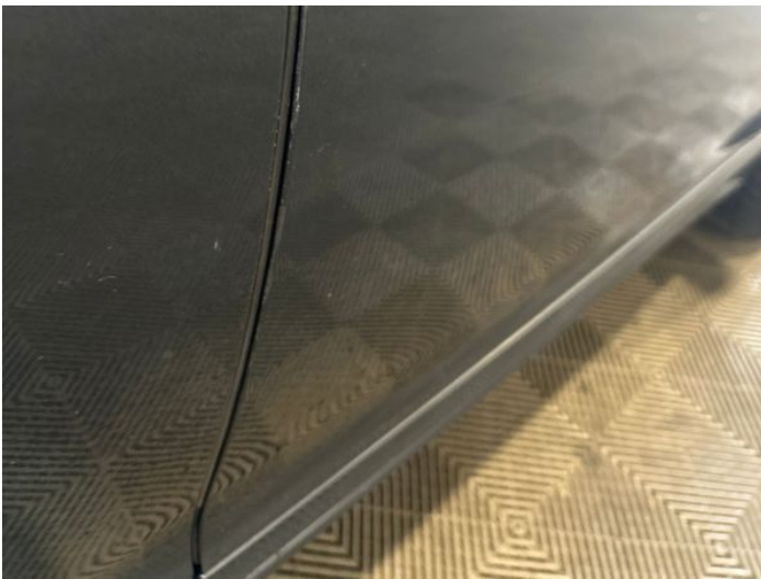
5: Door osf Chipped Edge Chip
