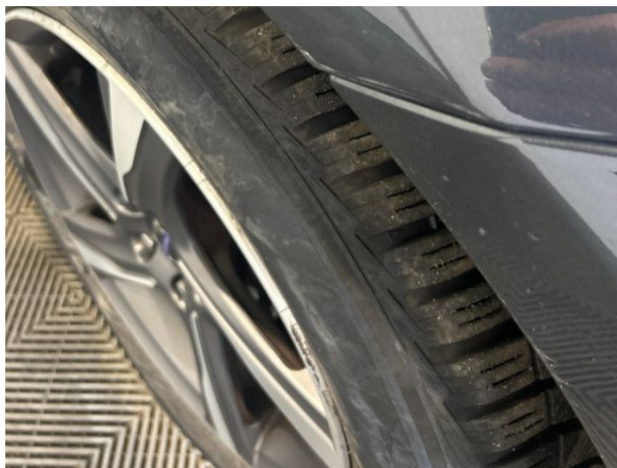
2: Wing osf Scratched Over 25mm Thru Paint
