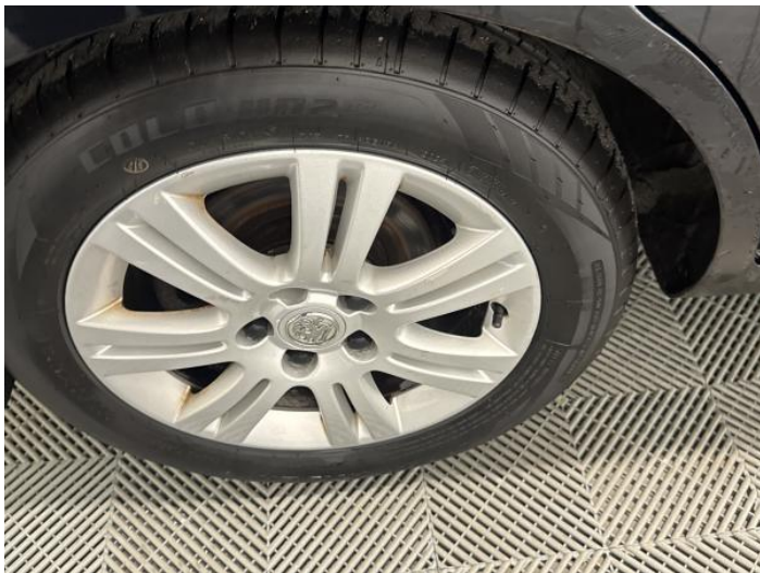
15: Wheel osr Scratched Over 50mm
