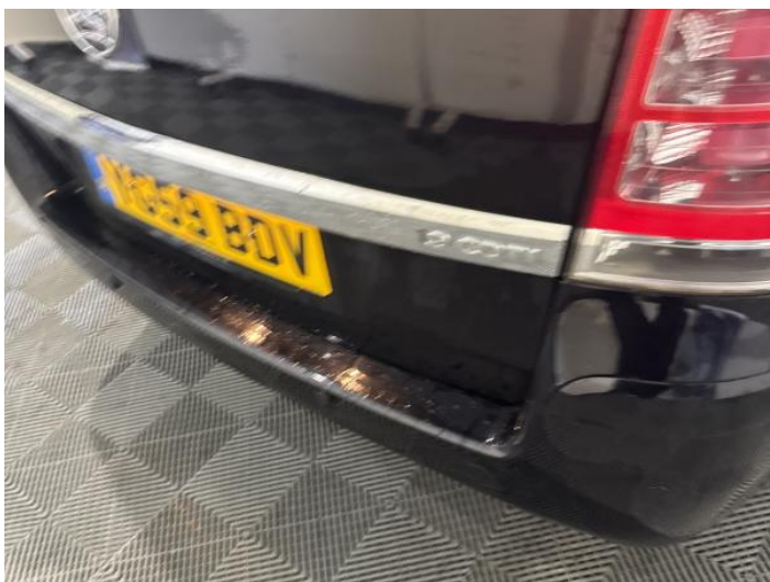
11: Bumper Rear Scratched 25 to 100mm Thru Paint
