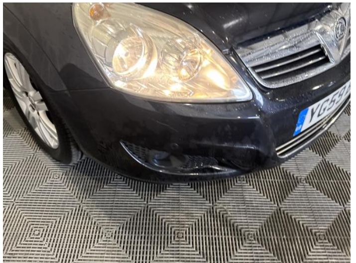
2: Bumper Front Scratched Over 100mm Thru Paint
