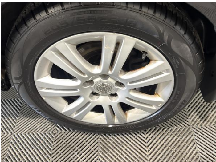
9: Wheel nsr Scratched Over 50mm
