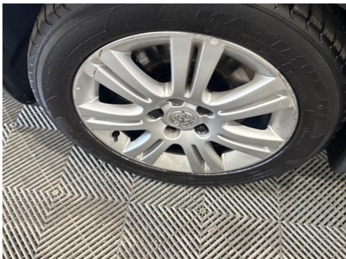
3: Wheel nsf Scratched Over 50mm
