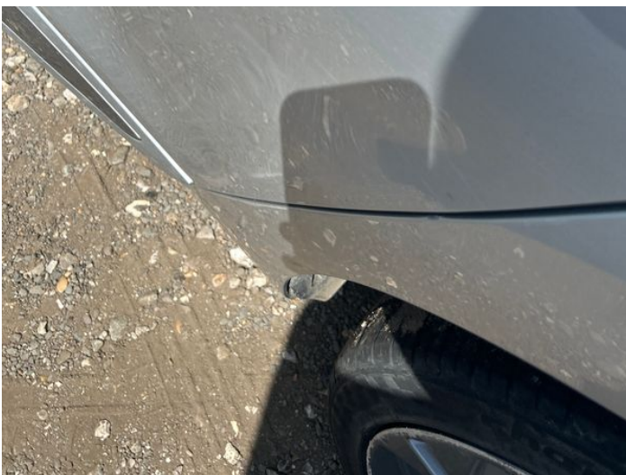
7: Door nsr Dented Over 30mm
