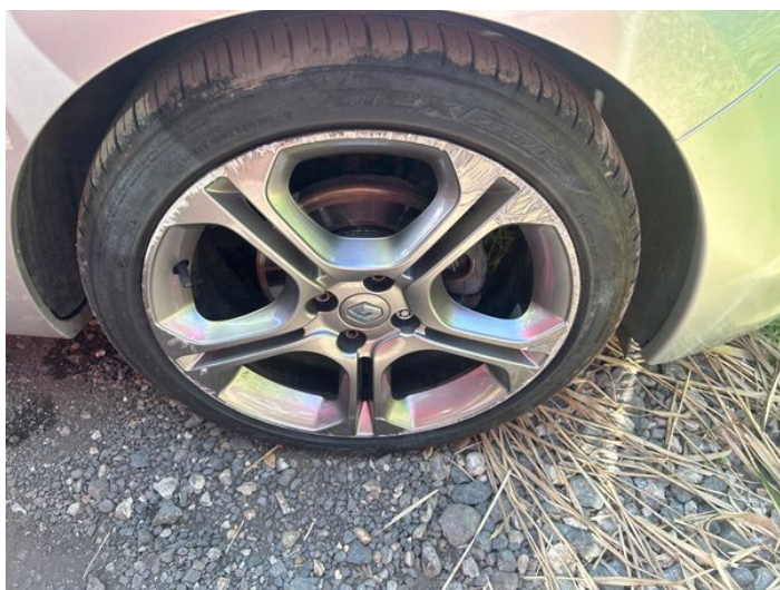
1: Wheel osf Scratched Over 50mm
