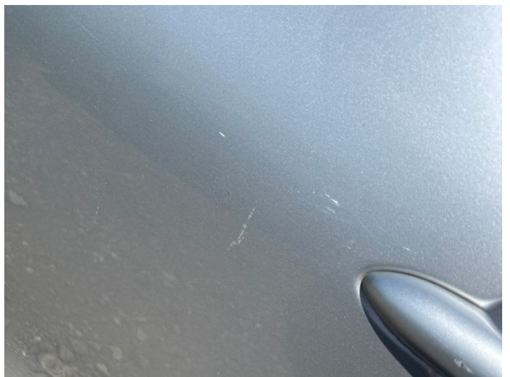
8: Door nsf Scratched UpTo 25mm Thru Paint
