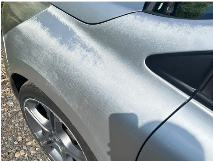
9: Wing nsf Poor Previous Repair Paint Flake
