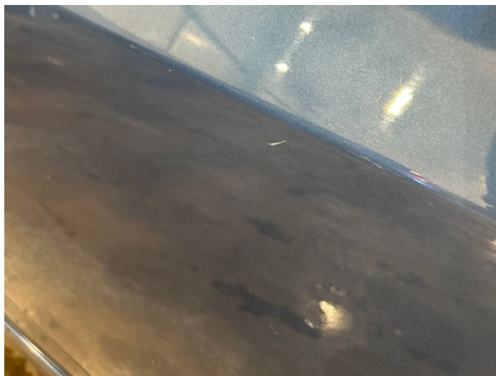
2: Door osf Chipped 1 To 5
