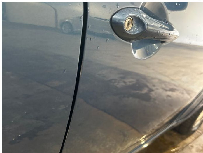
4: Door osf Chipped Edge Chip
