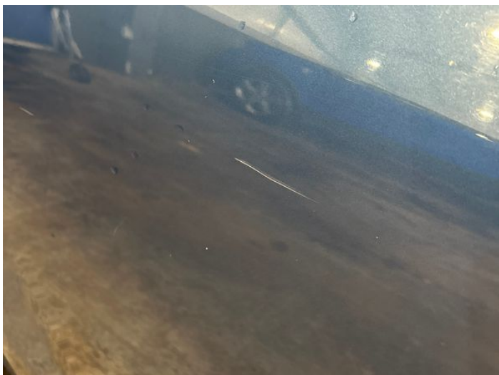
3: Door osr Scratched Over 25mm Thru Paint
