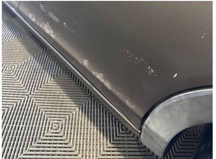
6: Door nsr Poor Previous Repair Paint Flake
