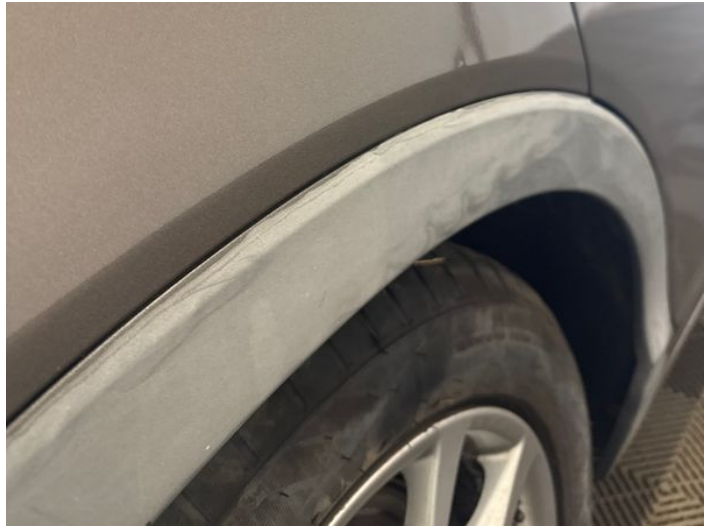
10: Qtr Panel osr Dented Between 10mm + 30mm
