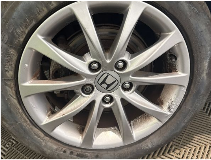
11: Wheel osr Scratched Over 50mm
