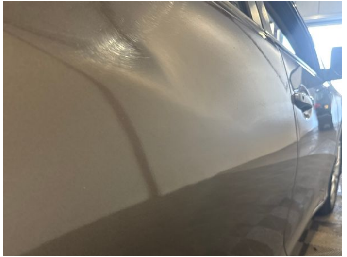
12: Door osr Poor Previous Repair Rippled UpTo 30%
