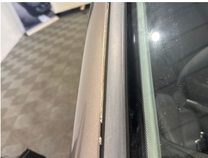
19: A Post os Scratched Over 25mm Thru Paint
