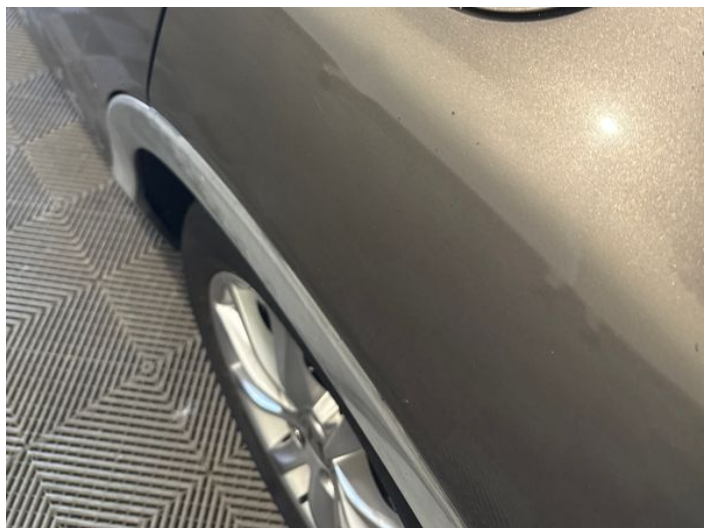
8: Qtr Panel nsr Dented Between 10mm + 30mm
