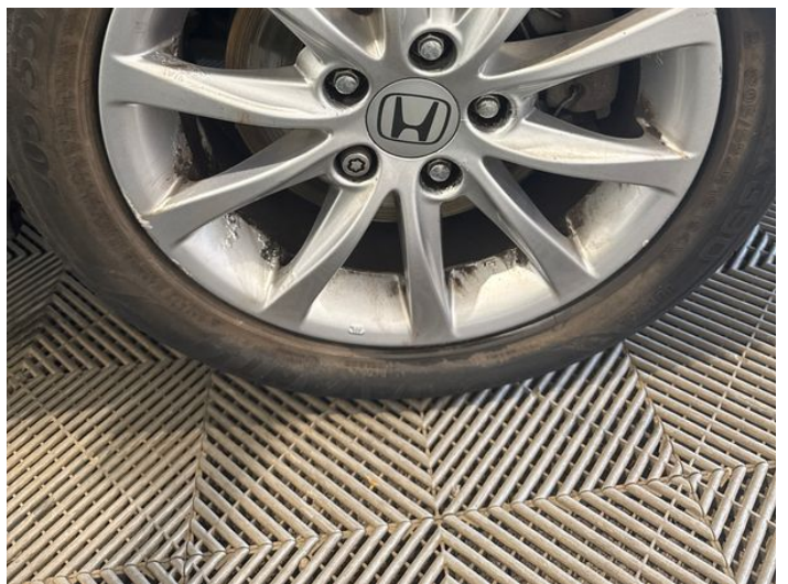
14: Wheel osf Scratched Over 50mm
