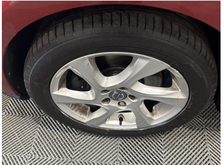
4: Wheel nsf Scratched Over 50mm
