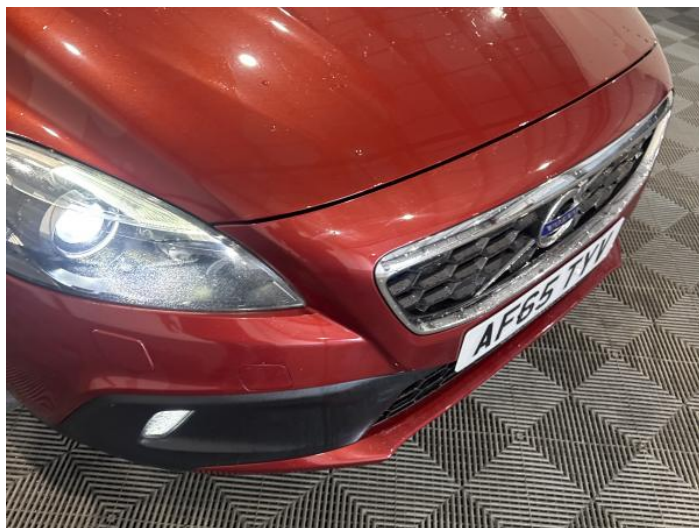
2: Bumper Front Chipped Multiple Chips
