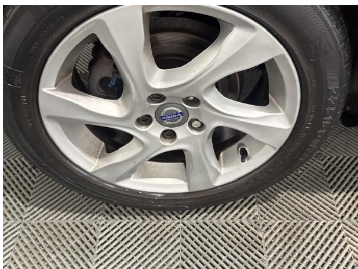
11: Wheel osr Scratched Up To 50mm
