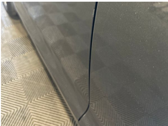
9: Door nsf Chipped Edge Chip
