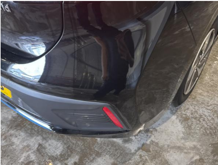
1: Bumper Rear Scratched Over 100mm Thru Paint
