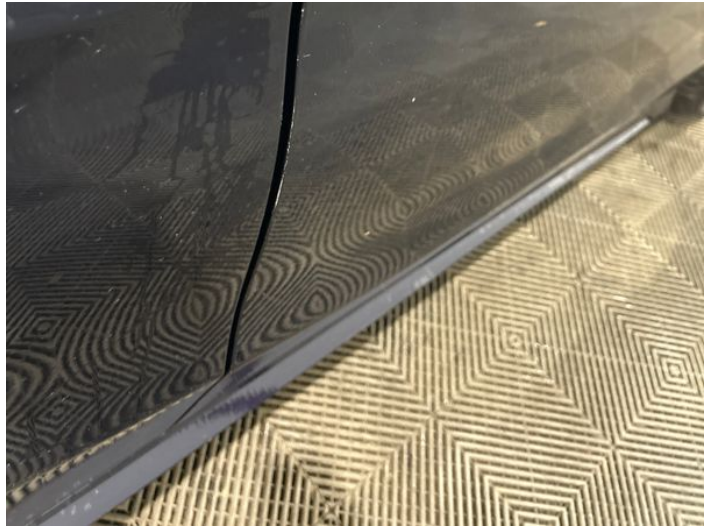
4: Door osf Chipped Edge Chip
