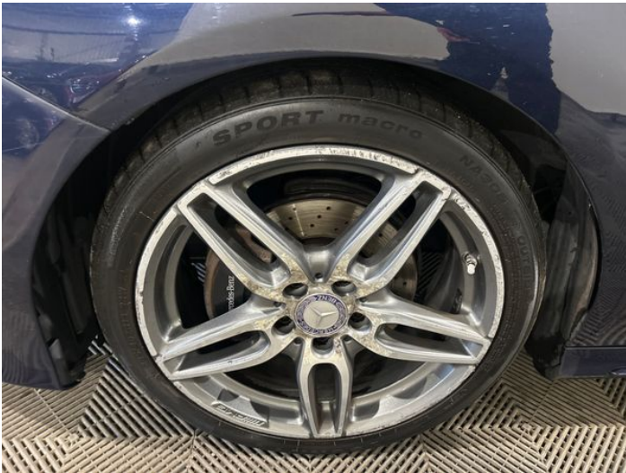
11: Wheel nsf Corroded Light
