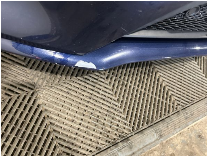
12: Bumper Front Poor Previous Repair Paint Flake
