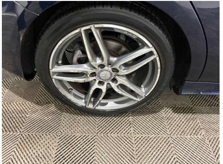
6: Wheel osr Corroded Light
