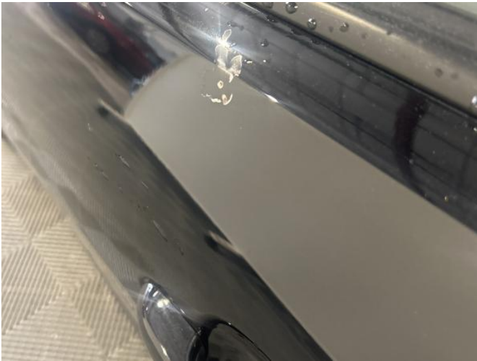
11: Door nsf Poor Previous Repair Paint Flake
