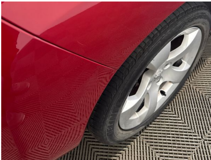
9: Qtr Panel osr Scratched UpTo 25mm Thru Paint
