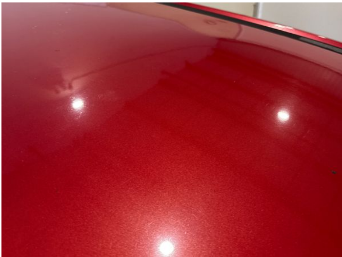
16: Roof Dented Over 30mm
