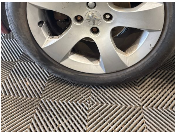
3: Wheel nsf Corroded Light
