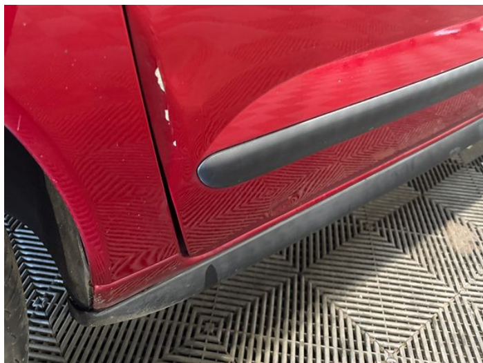
4: Door nsf Dented With Paint Damage
