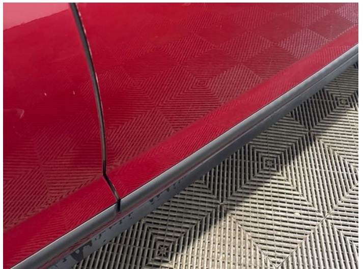
12: Door osf Scratched Over 25mm Thru Paint
