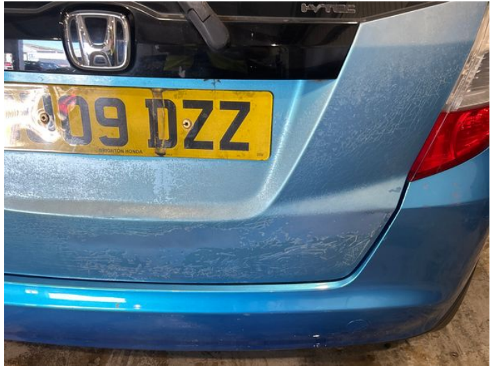
10: Tailgate Poor Previous Repair Poor Paint
