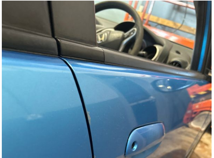
4: Door osf Chipped Edge Chip
