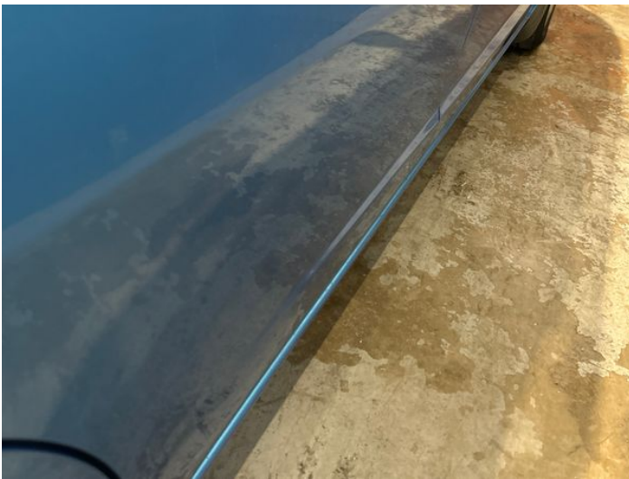
5: Door osr Dented Between 10mm + 30mm
