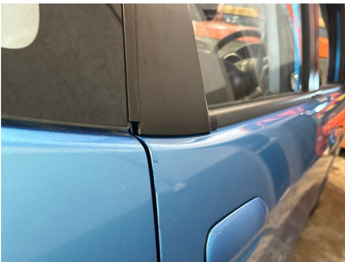
7: Door osr Chipped Edge Chip
