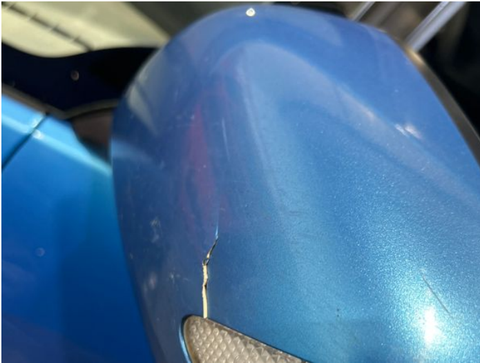
15: Door Mirror Assy nsf Broken Replace
