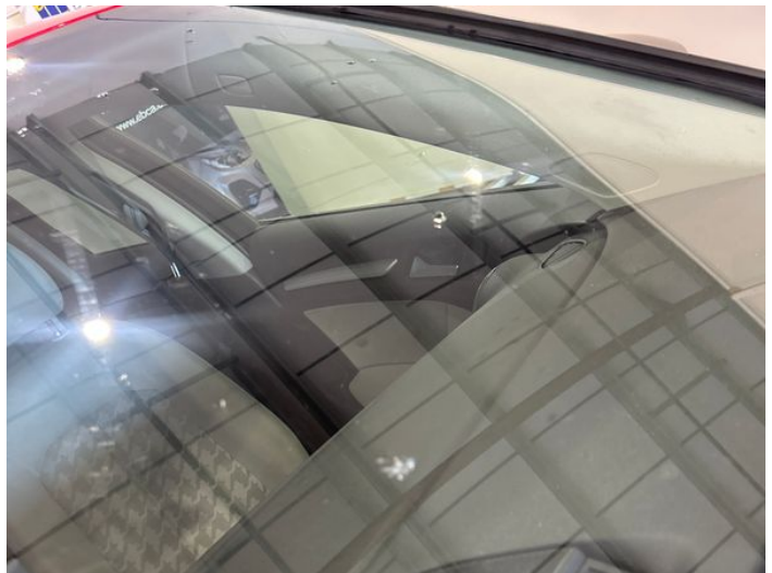
10: Screen Front Chipped UpTo 10mm
