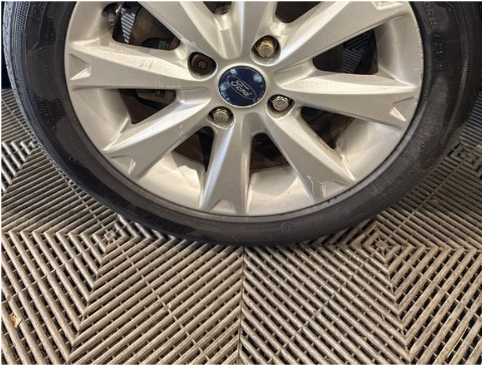
3: Wheel nsf Scratched Up To 50mm
