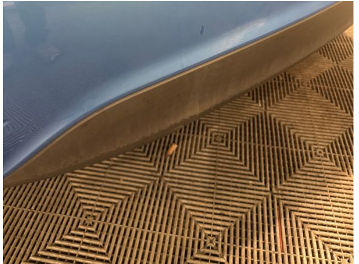
10: Bumper Rear Poor Previous Repair Poor Paint
