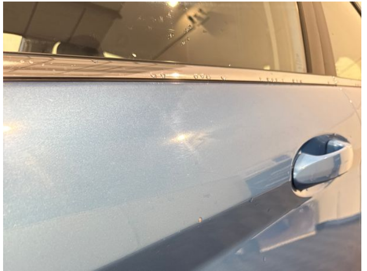
6: Door nsf Chipped Over 5mm
