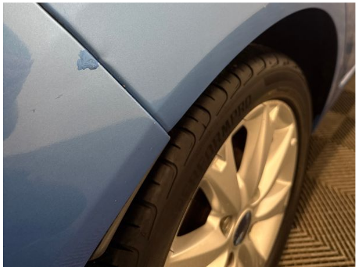
12: Qtr Panel osr Dented Between 10mm + 30mm
