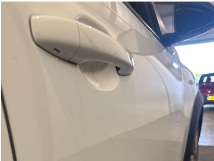
10: Door osf Dented Over 30mm
