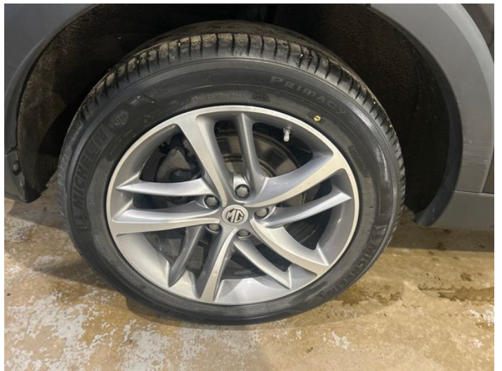
6: Wheel osr Corroded Light
