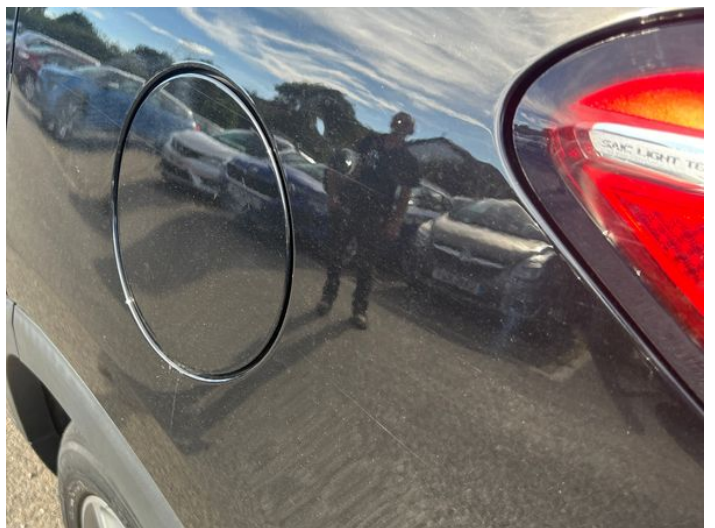
14: Qtr Panel nsr Dented Between 10mm + 30mm
