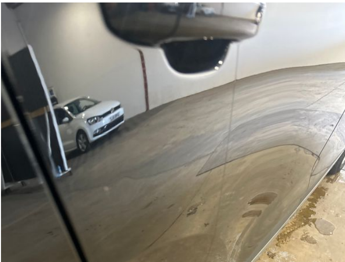
5: Door osr Dented Between 10mm + 30mm
