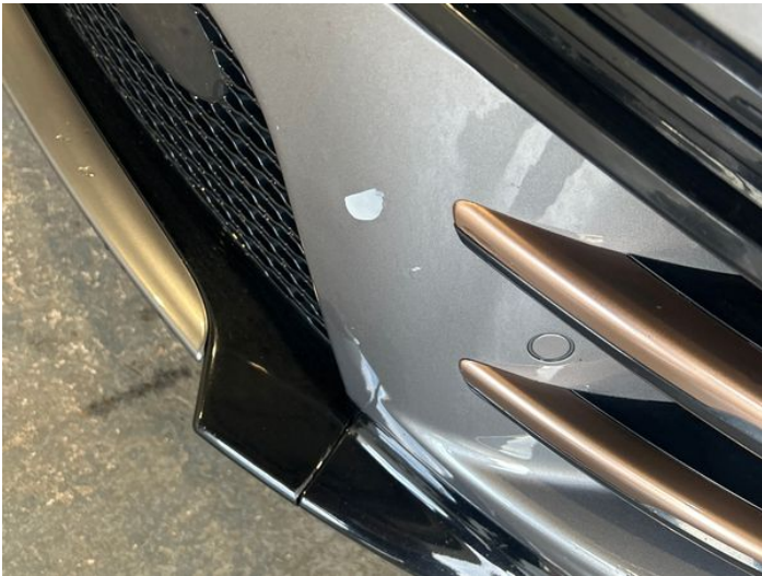
11: Bumper Front Poor Previous Repair Paint Flake
