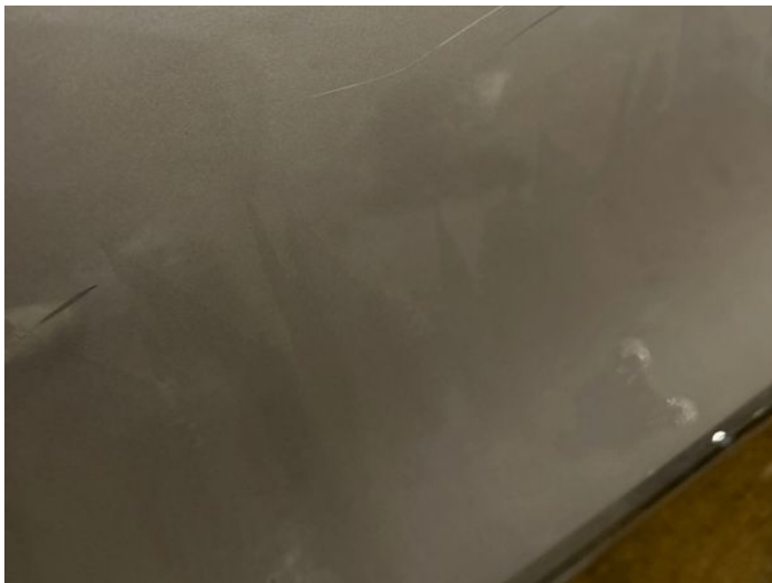
3: Door osr Scratched Over 25mm Thru Paint
