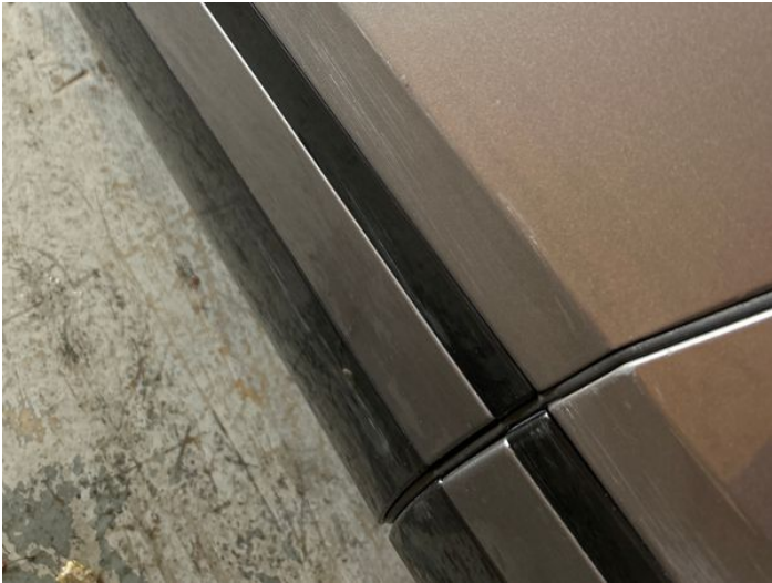
9: Door nsf Scratched Over 25mm Thru Paint
