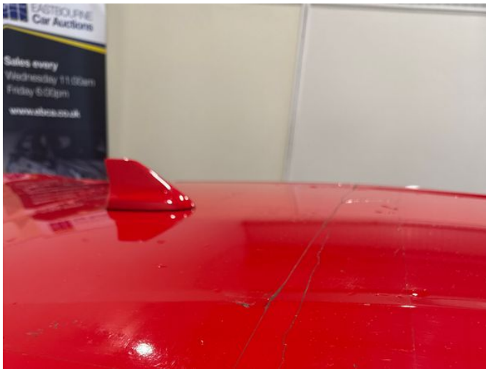
9: Roof Scratched Over 25mm Not Thru Paint
