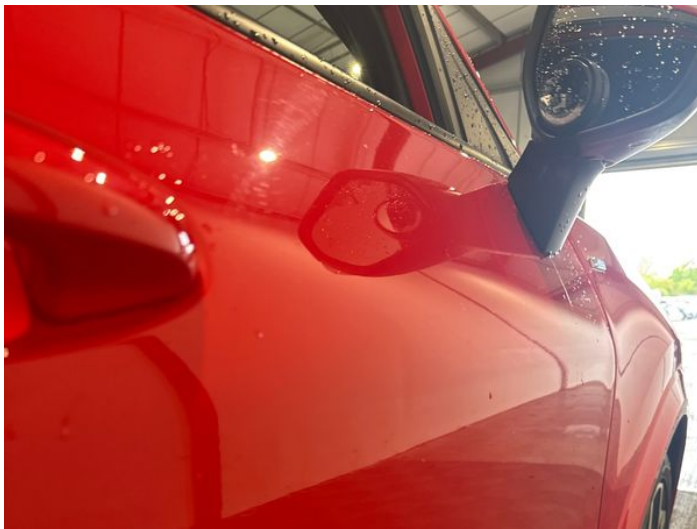
11: Door osf Dented Over 30mm
