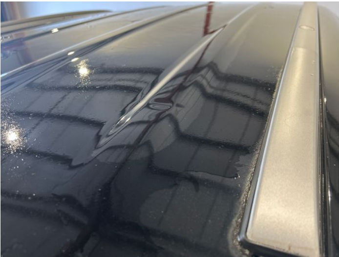
5: Roof Dented With Paint Damage
