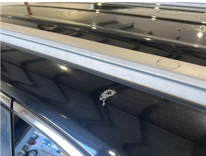
13: C Post ns Poor Previous Repair Paint Flake
