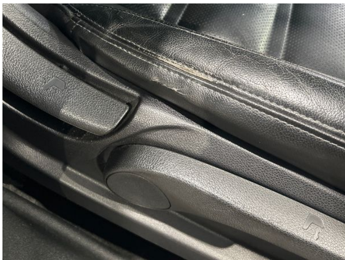
1: Seat Base Cover osf Torn UpTo 3mm
