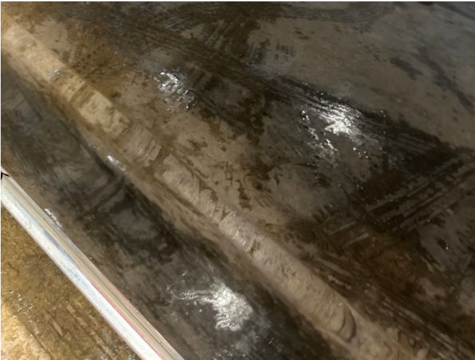
9: Door osf Chipped 1 To 5
