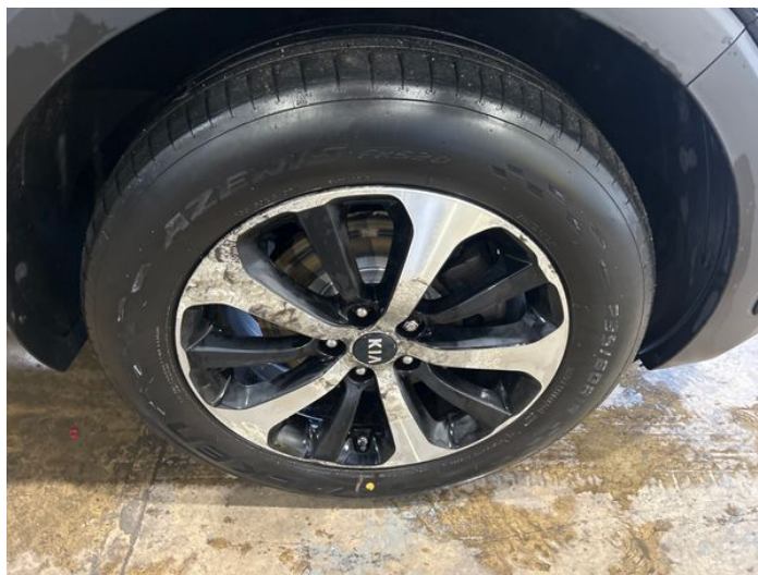
2: Wheel osf Corroded Light
