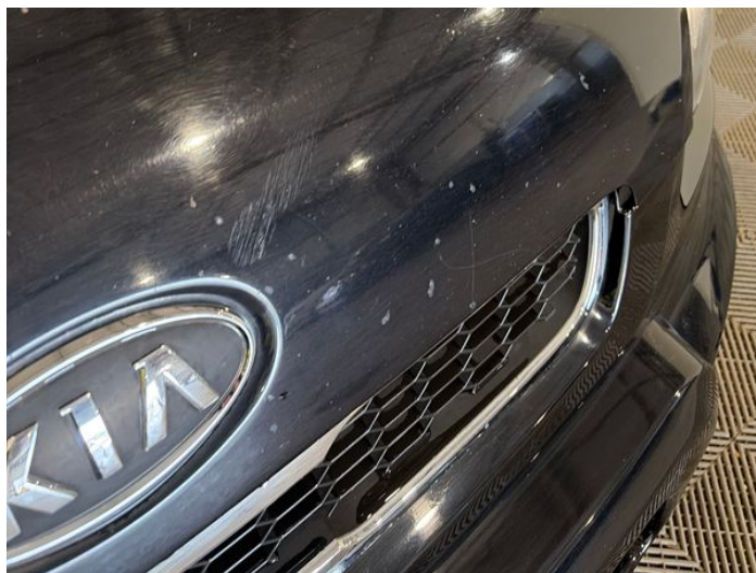
2: Bonnet Scratched Over 25mm Thru Paint
