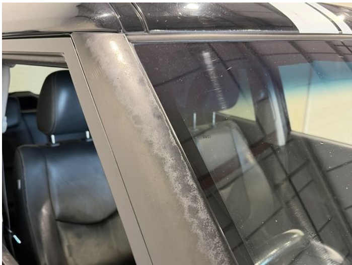
21: A Post os Scratched Over 25mm Thru Paint
