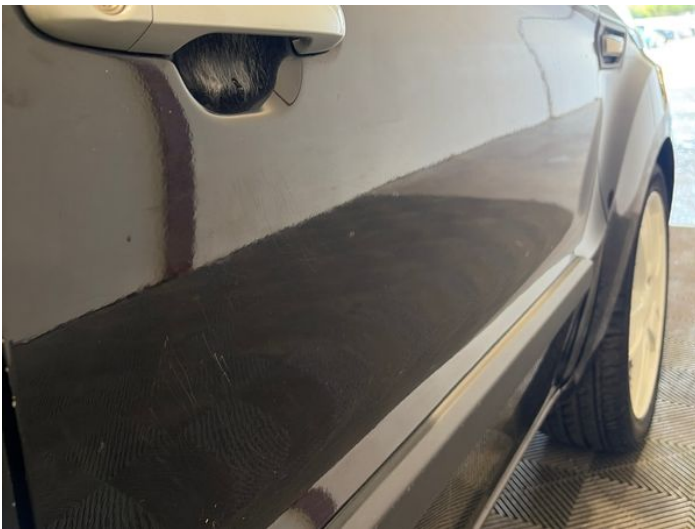
17: Door osf Dented Over 30mm
