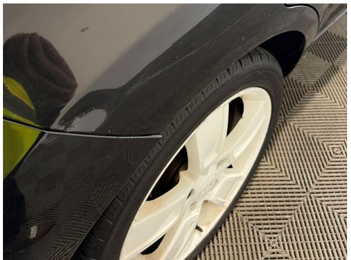
14: Qtr Panel osr Dented With Paint Damage
