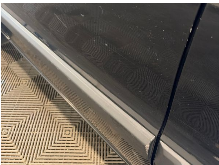
7: Door nsf Scratched Over 25mm Thru Paint
