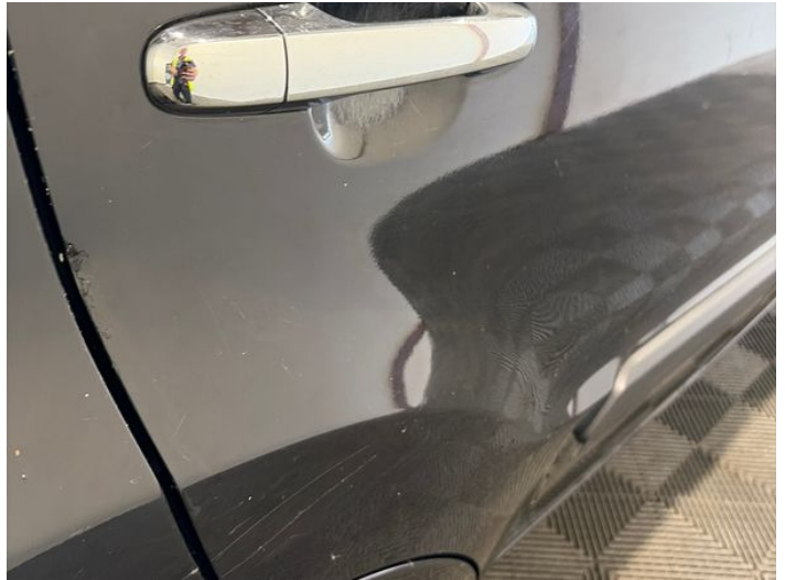
16: Door osr Dented With Paint Damage
