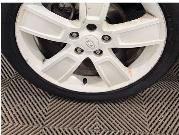
5: Wheel nsf Scratched Over 50mm
