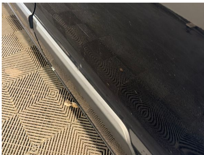
8: Door nsr Scratched Over 25mm Thru Paint
