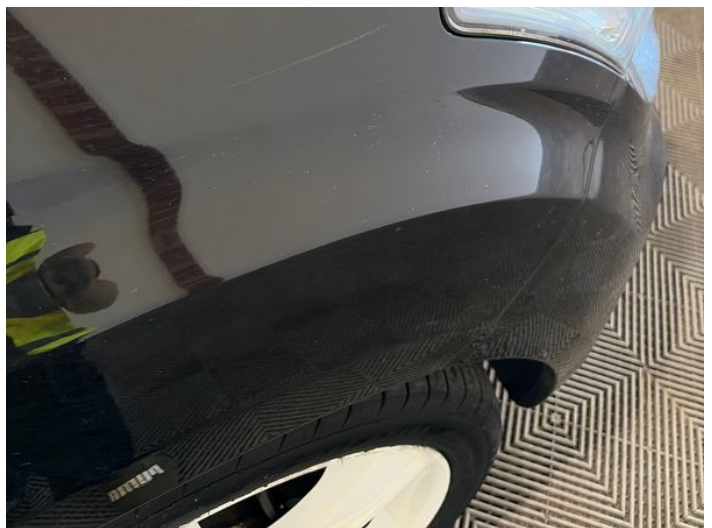
20: Wing osf Scratched Over 25mm Thru Paint
