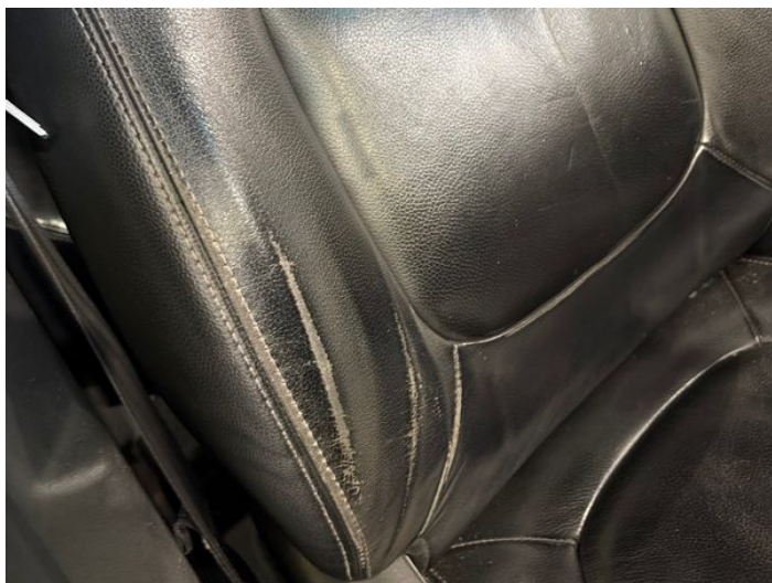
1: Seat Back Cover osf Scuffed Over 25mm
