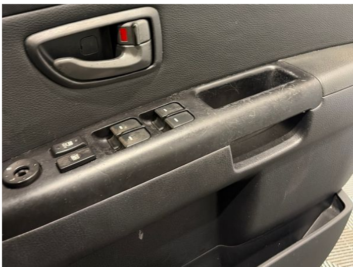
23: Door Pad osf Scuffed Over 25mm
