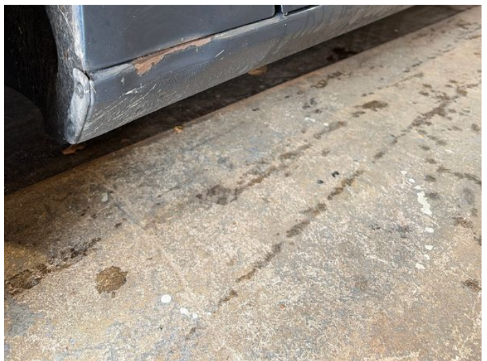
20: Sill ns Dented With Paint Damage
