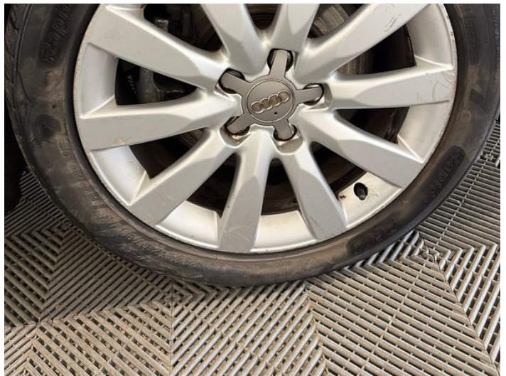
18: Wheel osf Scratched Over 50mm
