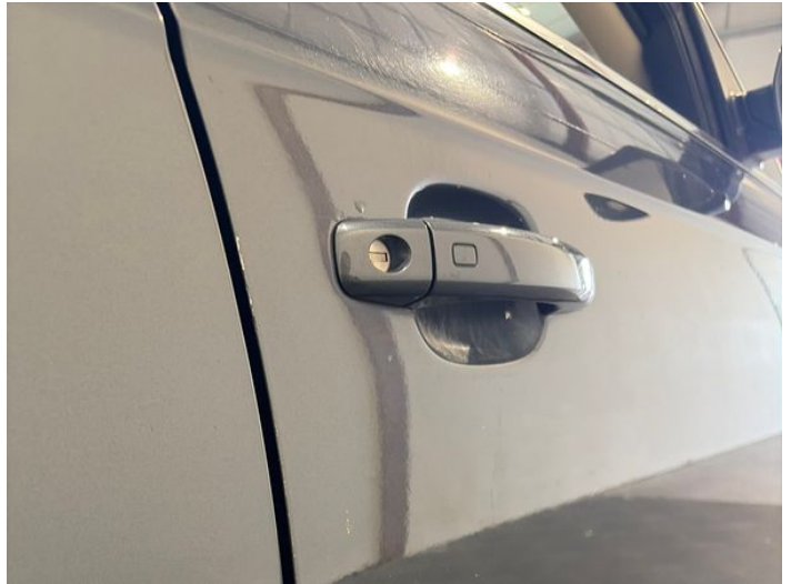
16: Door osf Scratched Over 25mm Thru Paint
