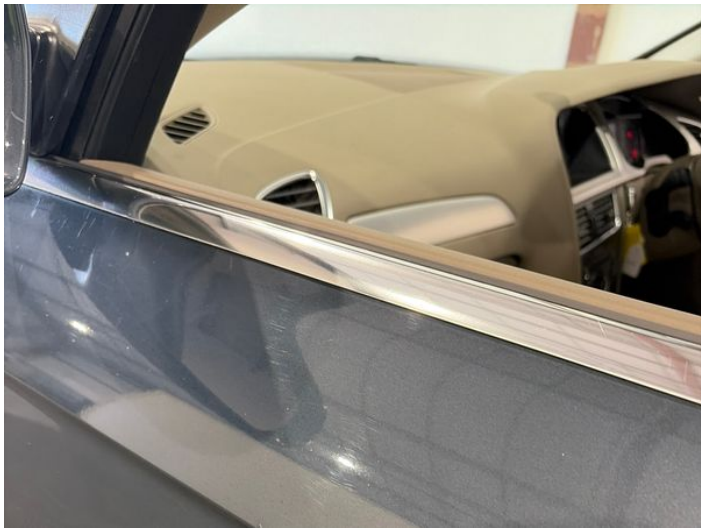
7: Door nsf Scratched UpTo 25mm Thru Paint
