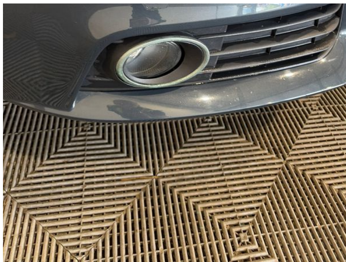
2: Bumper Front Poor Previous Repair Paint Flake
