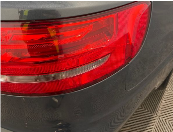
11: Lamp osr Broken Replace
