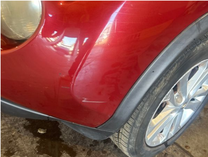
15: Bumper Front Scratched Over 100mm Thru Paint
