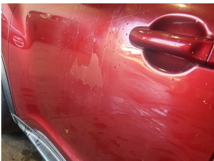
13: Door nsf Dented With Paint Damage
