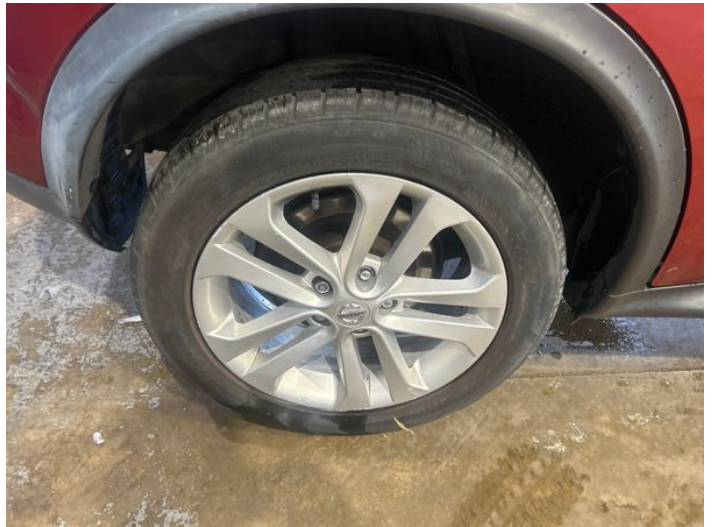
6: Wheel osr Scratched Over 50mm
