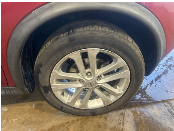
1: Wheel osf Scratched Over 50mm
