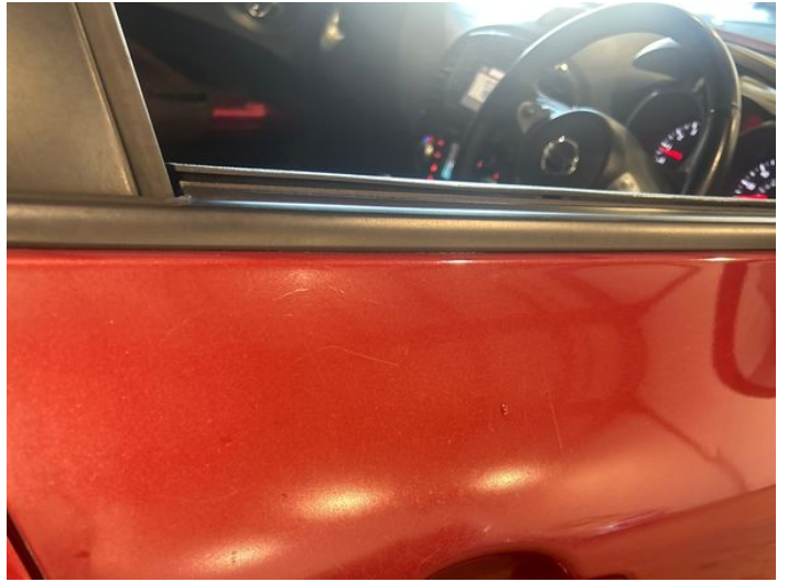
4: Door osf Poor Previous Repair Poor Paint
