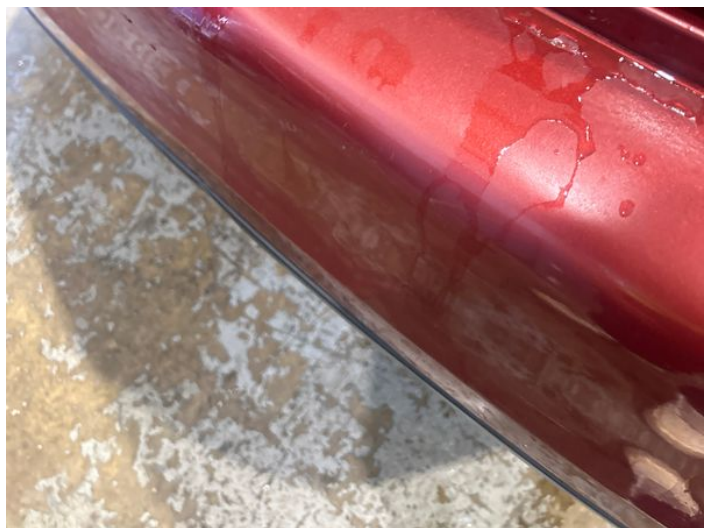
8: Bumper Rear Poor Previous Repair Paint Flake
