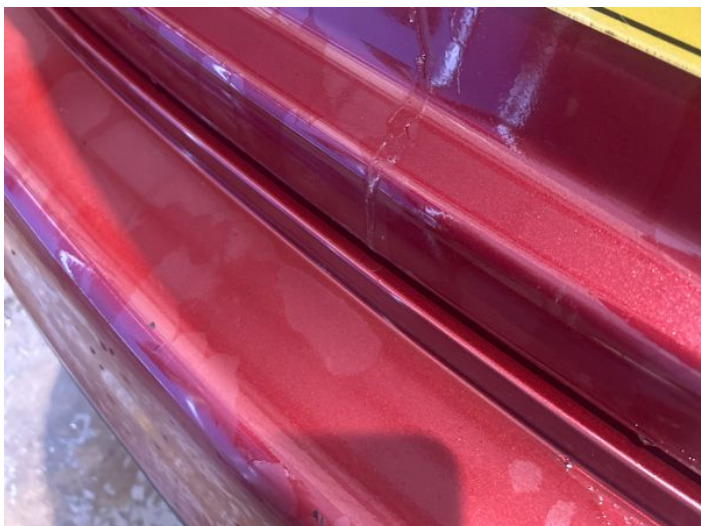
9: Tailgate Poor Previous Repair Poor Paint
