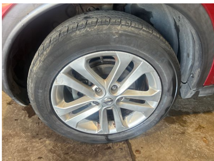
14: Wheel nsf Scratched Over 50mm
