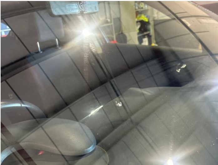
17: Screen Front Chipped UpTo 10mm
