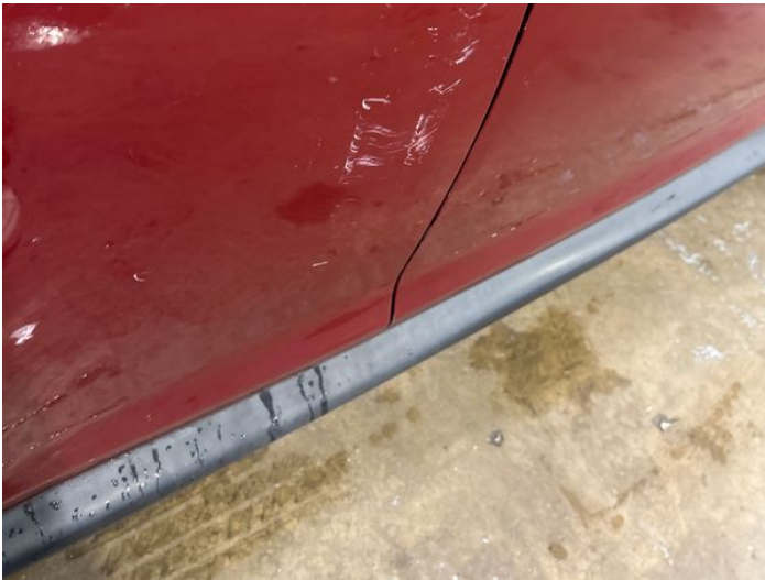
5: Door osr Dented With Paint Damage
