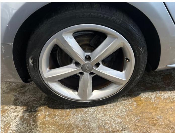
7: Wheel osr Scratched Over 50mm
