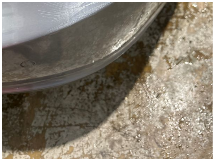
8: Bumper Rear Poor Previous Repair Paint Flake
