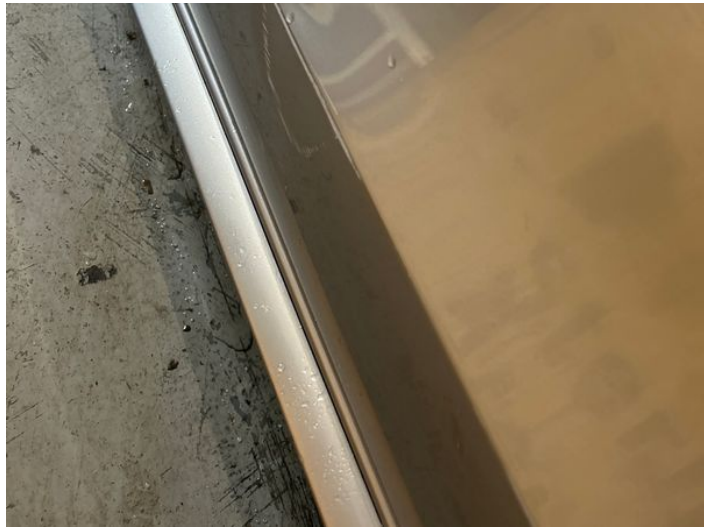
12: Door nsf Dented With Paint Damage
