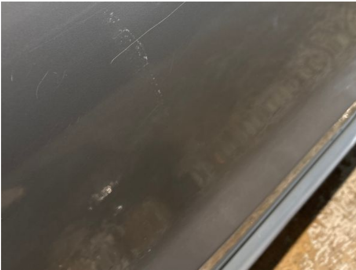
5: Door osr Scratched Over 25mm Thru Paint
