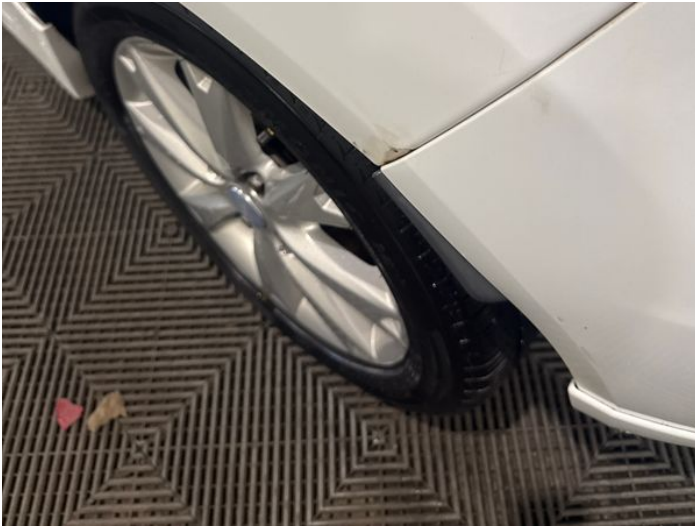
9: Qtr Panel nsr Dented With Paint Damage
