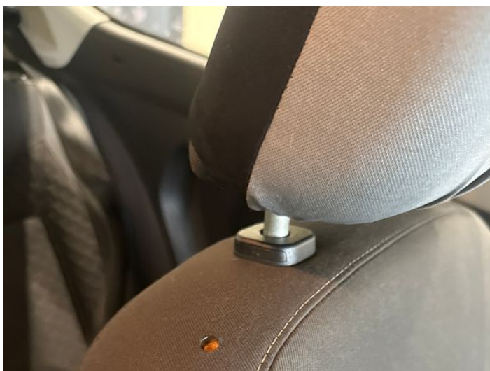
1: Seat Back Cover nsf Burn Over 3mm
