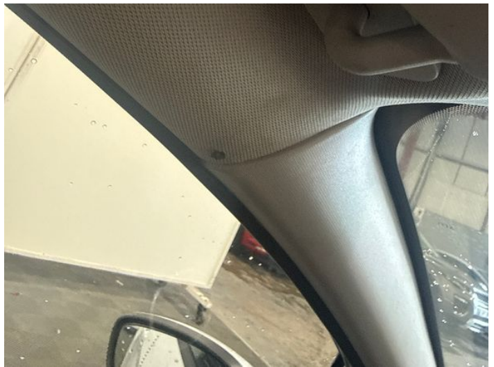
24: Roof Lining Burn Over 3mm
