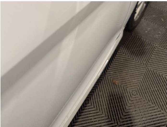
17: Door osf Dented Between 10mm + 30mm
