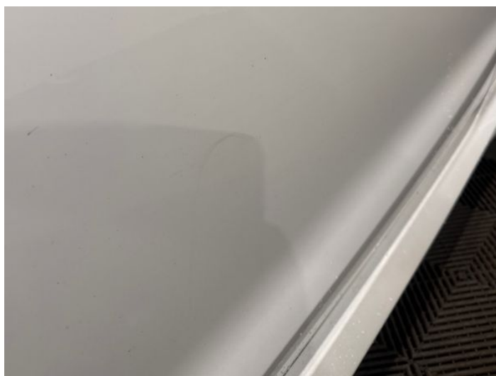
8: Door nsf Scratched Over 25mm Thru Paint
