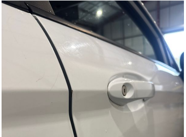
16: Door osf Chipped Edge Chip
