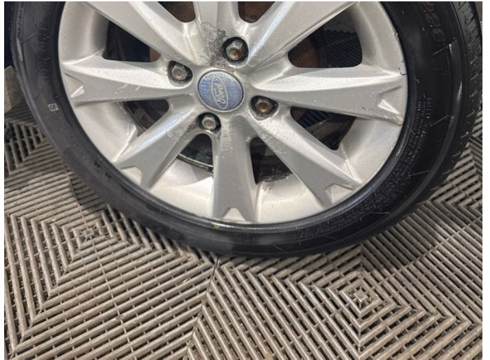
10: Wheel nsr Scratched Over 50mm
