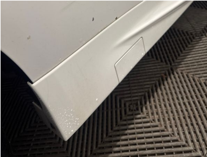
15: Qtr Panel osf Chipped Over 5mm
