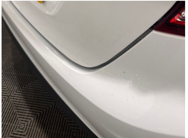
12: Tailgate Scratched Over 25mm Thru Paint
