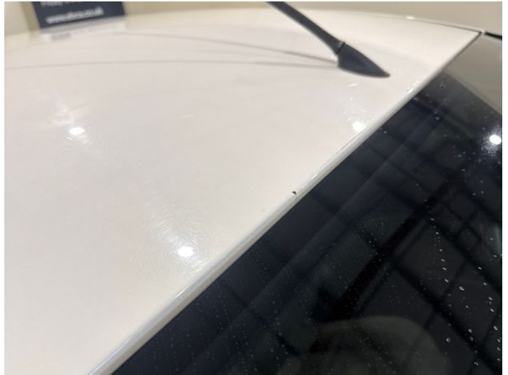
22: Roof Chipped Edge Chip
