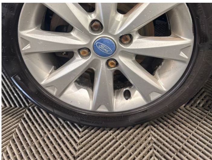
7: Wheel nsf Scratched Over 50mm
