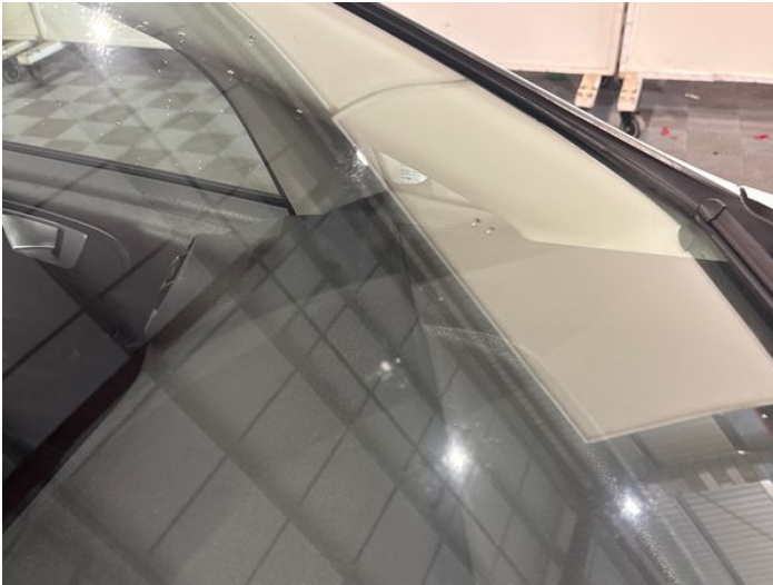
21: Screen Front Cracked Replace
