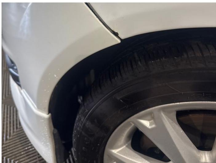
5: Wing nsf Dented Between 10mm + 30mm
