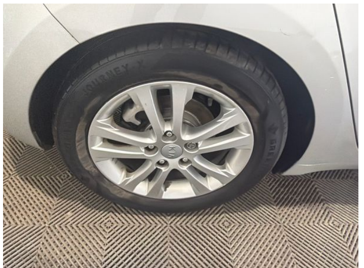
8: Wheel osr Scratched Up To 50mm
