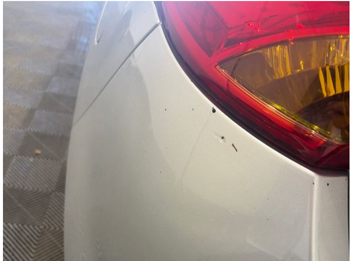
10: Bumper Rear Poor Previous Repair Poor Paint
