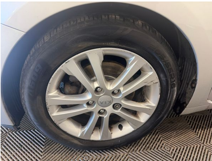
17: Wheel nsf Scratched Over 50mm
