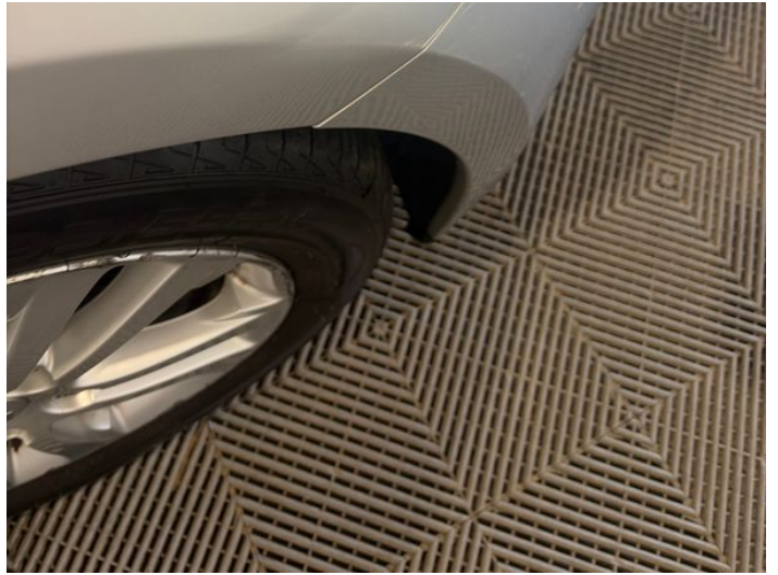
4: Door osf Dented Over 30mm
