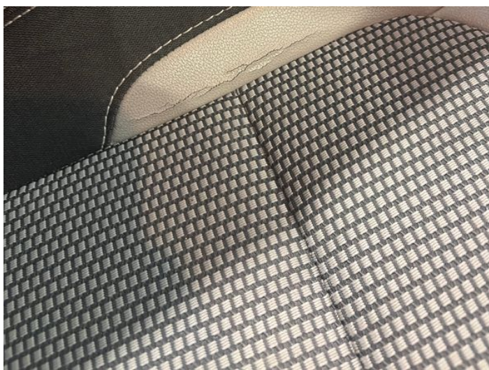
1: Seat Base Cover nsf Torn Over 3mm
