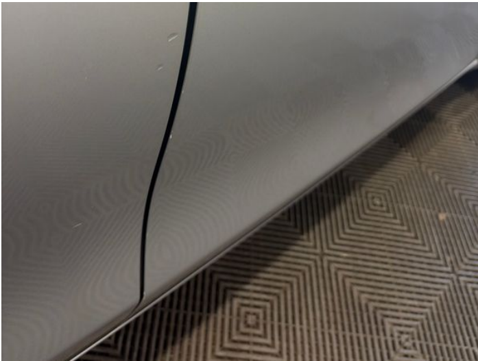
5: Door osf Chipped Edge Chip
