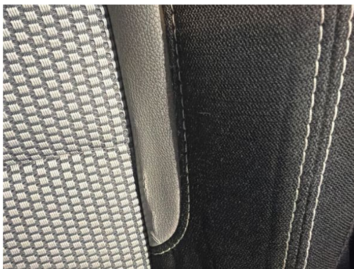
2: Seat Base Cover osf Torn UpTo 3mm
