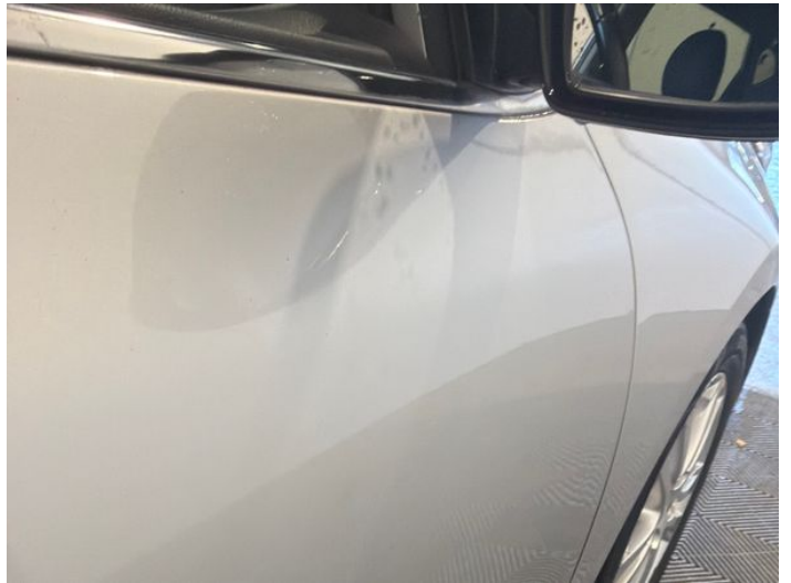
6: Door osf Dented Between 10mm + 30mm
