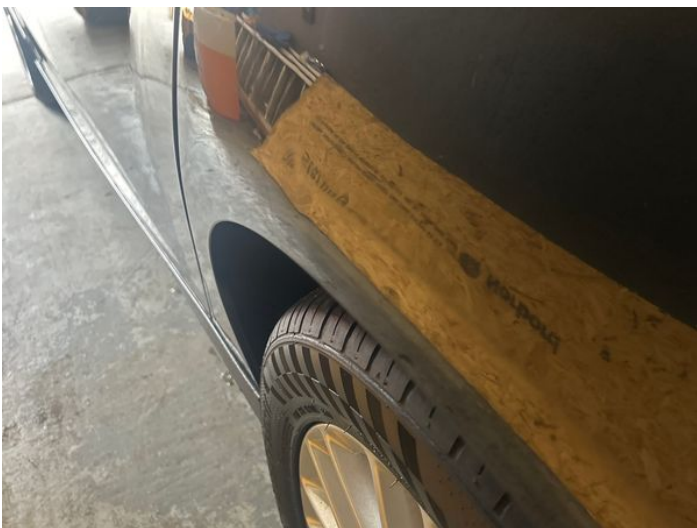
7: Qtr Panel nsr Dented Between 10mm + 30mm
