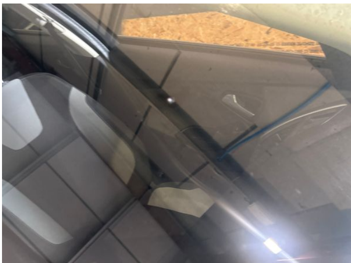
15: Screen Front Chipped UpTo 10mm
