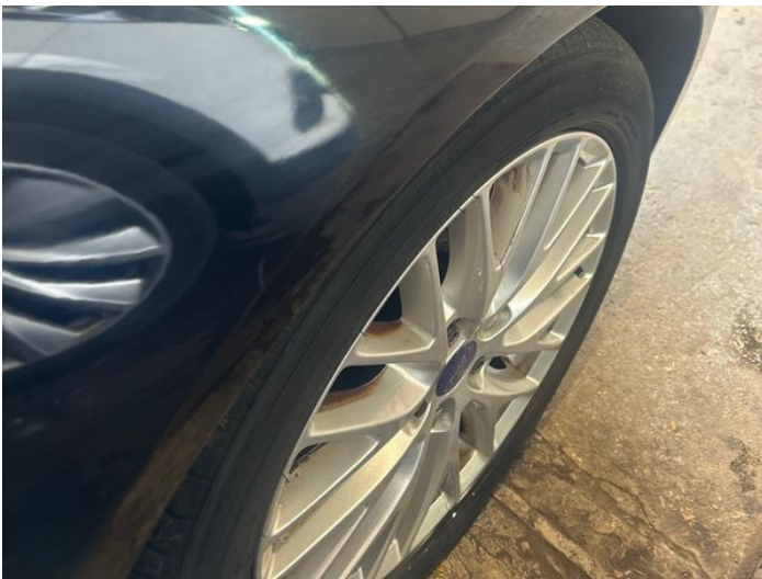
1: Wing osf Poor Previous Repair Poor Paint
