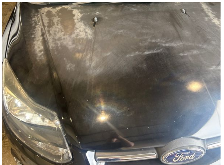
14: Bonnet Poor Previous Repair Paint Flake
