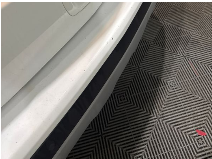
9: Bumper Rear Scratched 25 to 100mm Thru Paint
