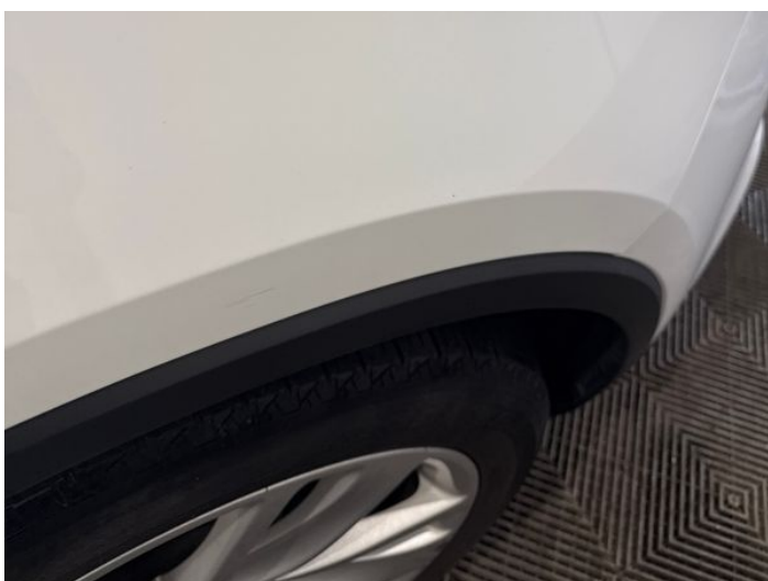
17: Wing osf Scratched UpTo 25mm Thru Paint
