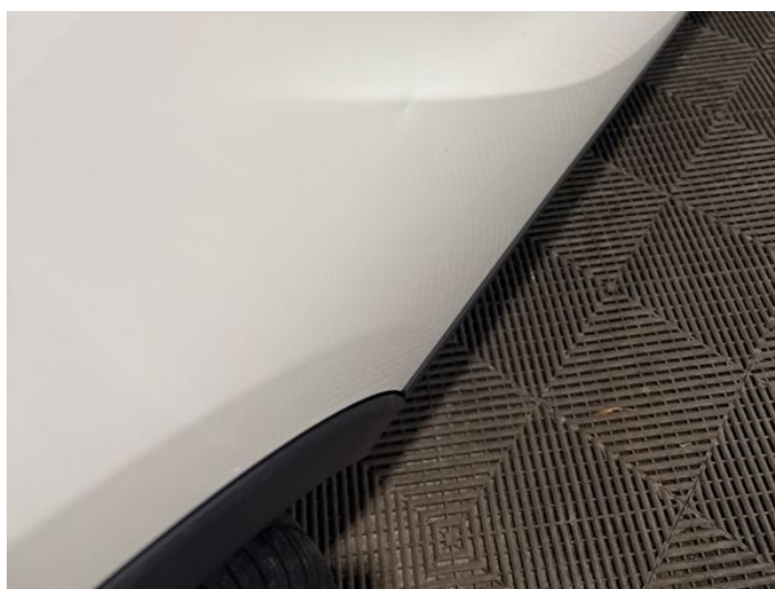
12: Door osr Dented Between 10mm + 30mm
