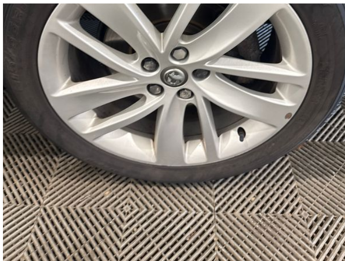
16: Wheel osf Scratched Up To 50mm
