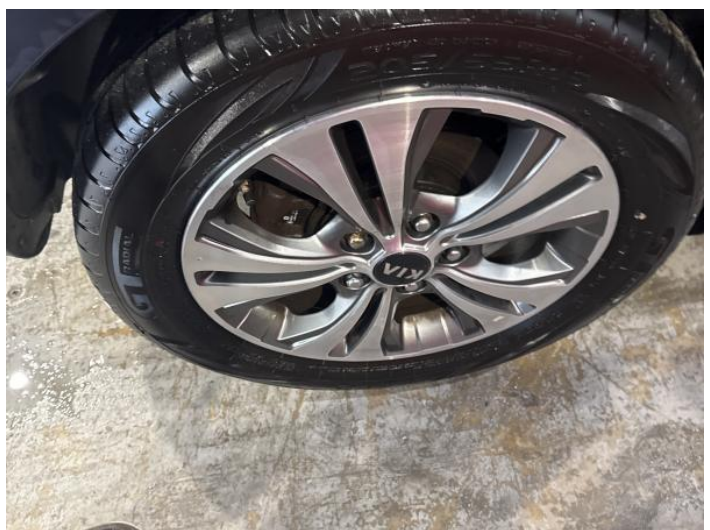
20: Wheel osr Scratched Up To 50mm
