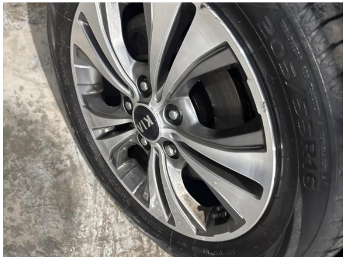
18: Wheel nsf Scratched Up To 50mm
