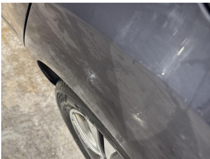
13: Qtr Panel nsr Dented Over 30mm
