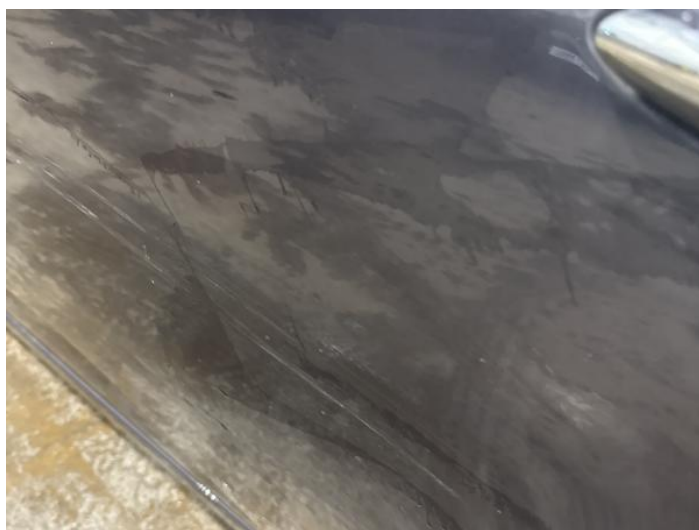
14: Door nsr Scratched Over 25mm Thru Paint
