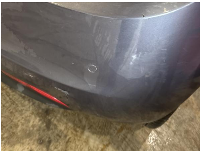
11: Bumper Rear Cracked UpTo 25mm
