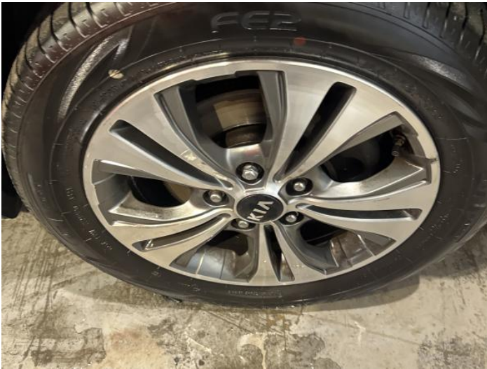
5: Wheel osf Scratched Over 50mm
