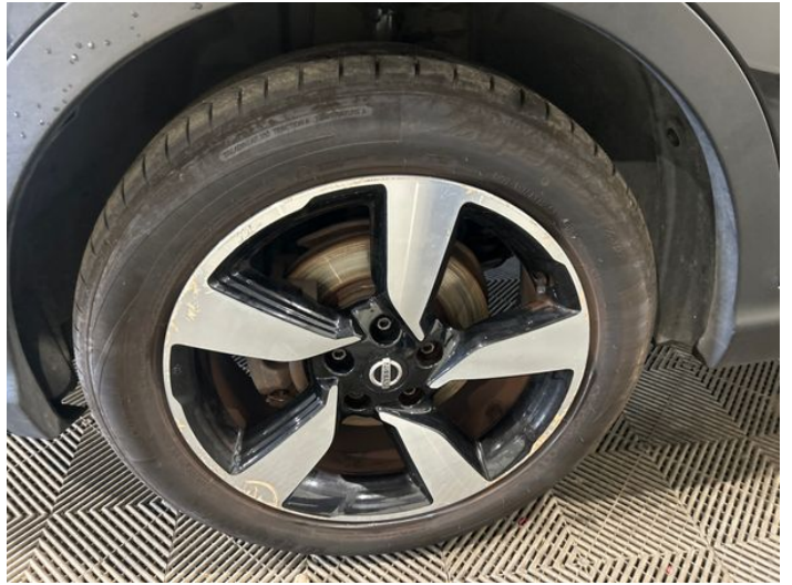
10: Wheel nsf Corroded Light
