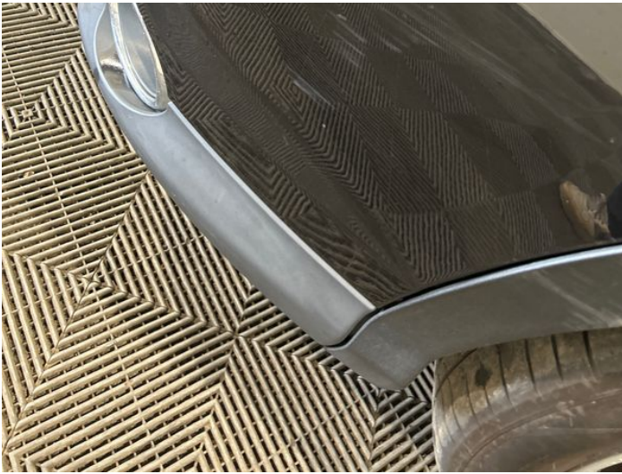
11: Bumper Front Scratched 25 to 100mm Thru Paint
