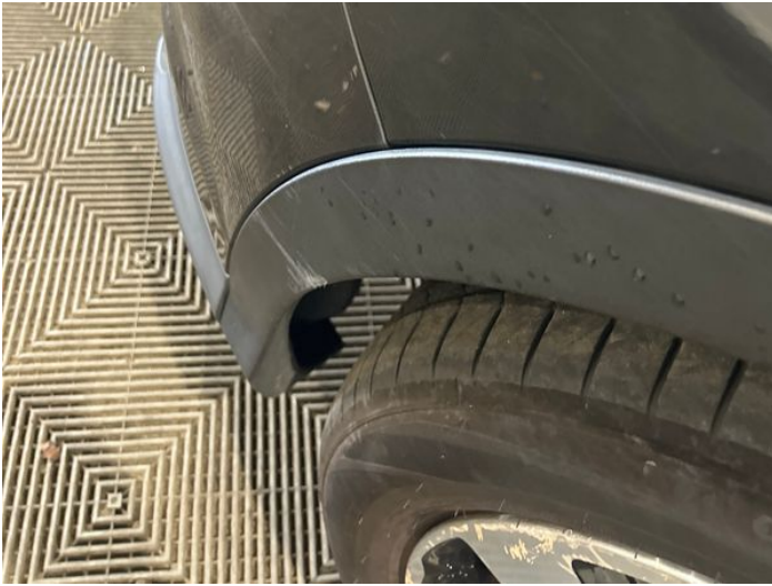
9: Wing nsf Dented Over 30mm
