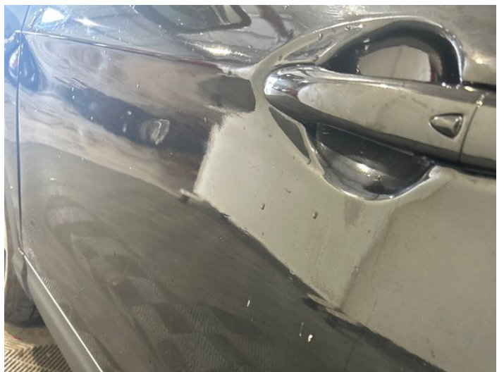
8: Door nsf Poor Previous Repair Poor Paint
