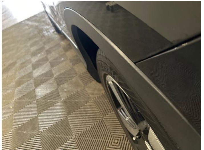
6: Qtr Panel nsr Dented Between 10mm + 30mm
