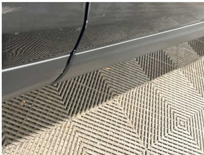
2: Door osf Chipped Edge Chip
