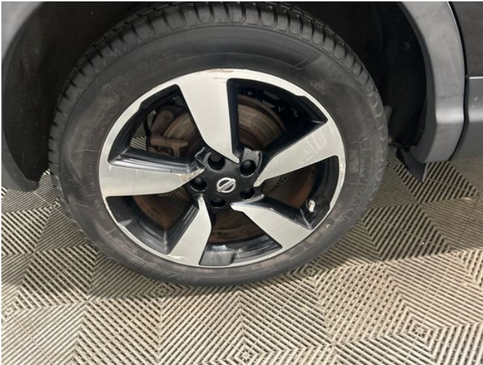
3: Wheel osr Corroded Light
