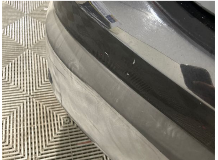
4: Bumper Rear Chipped 1 To 5
