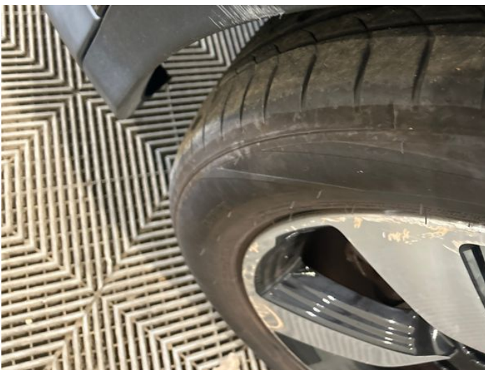
13: Wing Front Arch Extension ns Scuffed (Unpainted) UpTo 100mm
