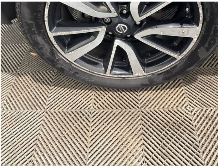
11: Wheel osr Scratched Over 50mm
