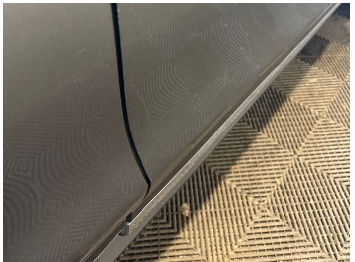
14: Door osf Chipped Edge Chip
