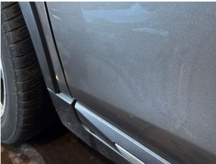
5: Door nsf Scratched Over 25mm Thru Paint
