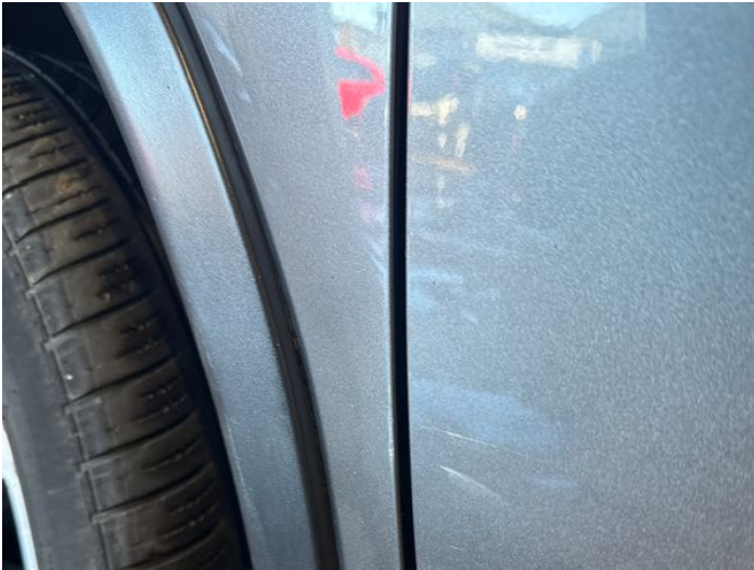
3: Wing nsf Scratched UpTo 25mm Thru Paint
