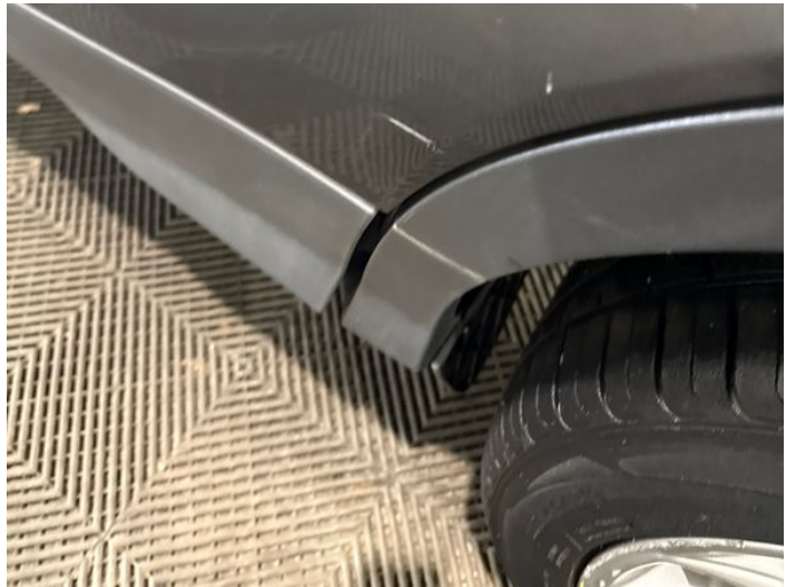
6: Door osr Scratched Over 25mm Thru Paint
