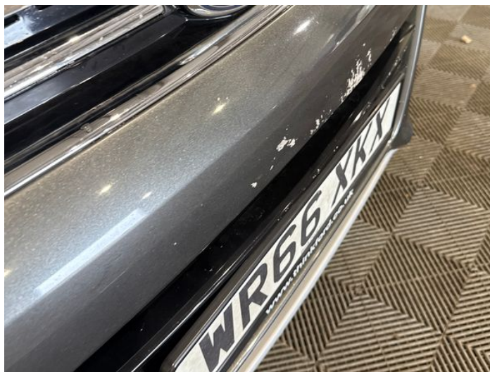
2: Bumper Front Poor Previous Repair Paint Flake
