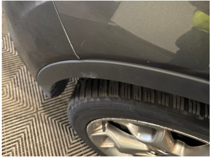
4: Wing nsf Scratched UpTo 25mm Thru Paint
