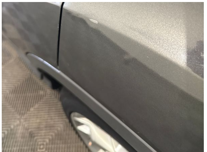
8: Qtr Panel nsr Dented Between 10mm + 30mm
