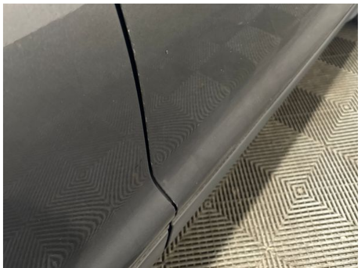
14: Door osf Chipped Edge Chip
