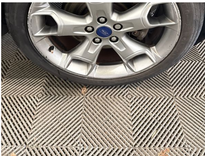
17: Wheel osf Scratched Over 50mm
