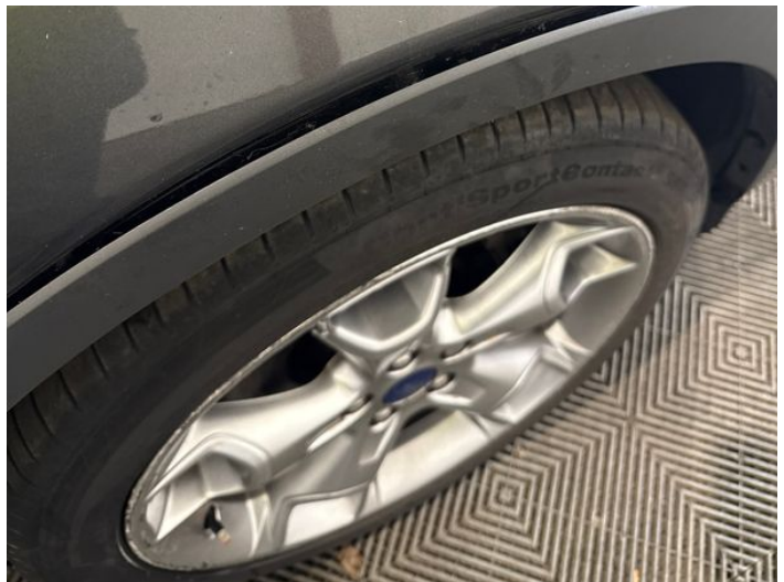
16: Wing Front Arch Extension os Scuffed (Unpainted) Over 100mm
