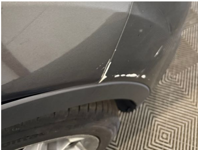
15: Wing osf Scratched Over 25mm Thru Paint
