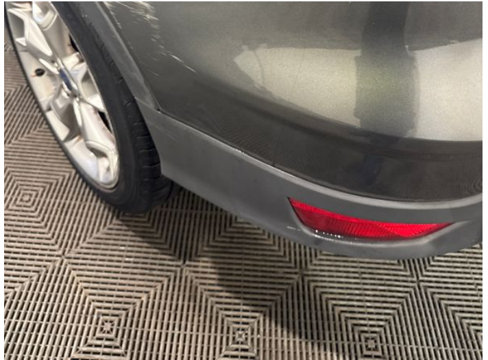
10: Bumper Rear Scratched Over 100mm Thru Paint
