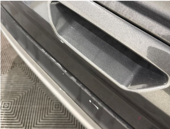
11: Tailgate Trim Panel Scratched (Painted) UpTo 25mm Thru Paint
