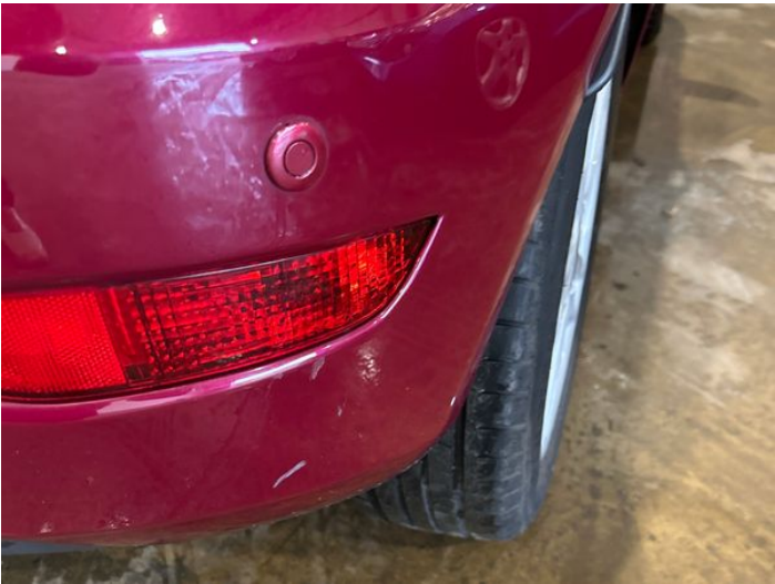
6: Bumper Rear Scratched 25 to 100mm Thru Paint
