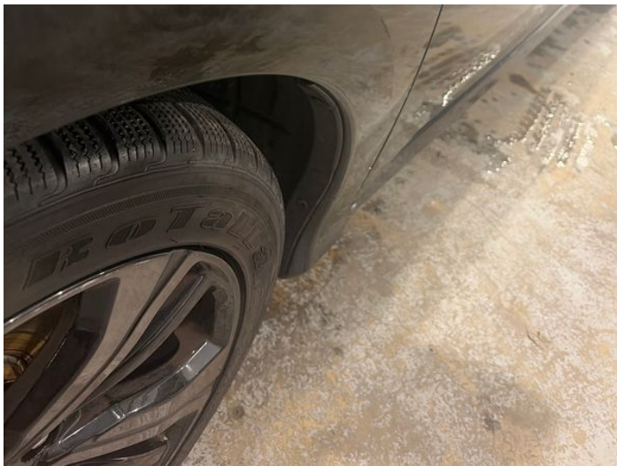
11: Wing nsf Dented 2 Or Less UpTo 10mm
