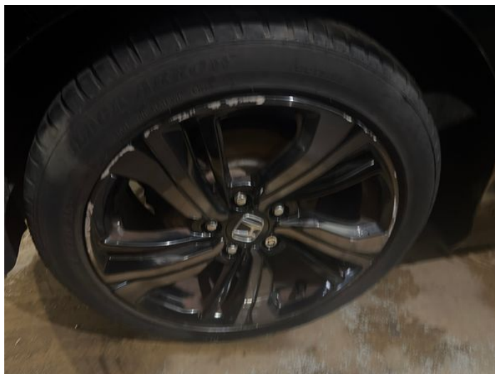
4: Wheel osr Scratched Over 50mm
