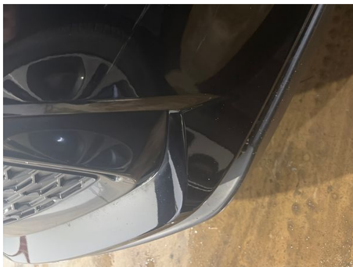
6: Bumper Rear Scratched Over 100mm Thru Paint
