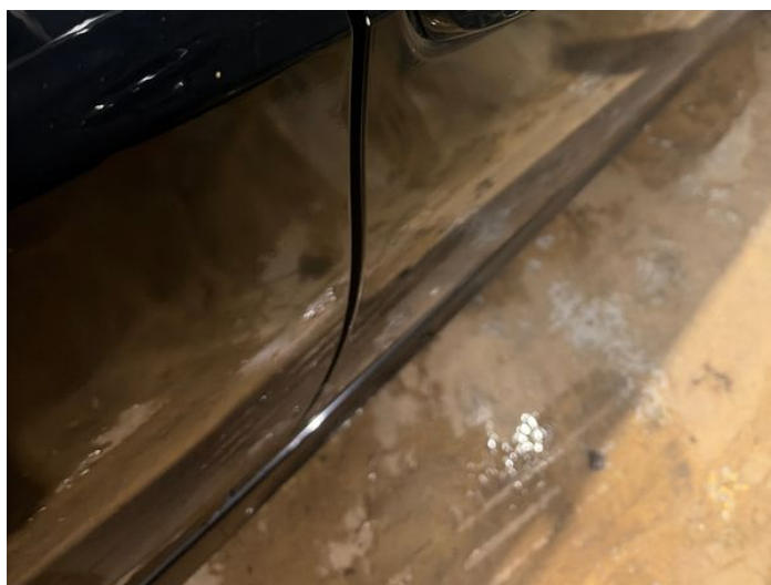
2: Door osf Chipped Edge Chip
