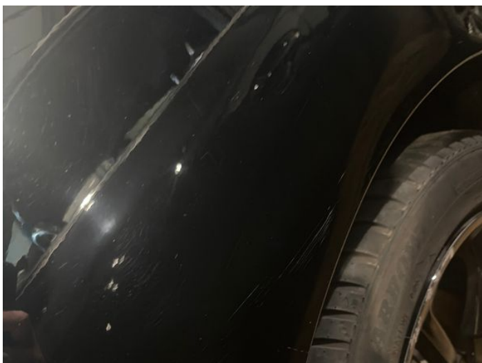
5: Qtr Panel osr Scratched Over 25mm Thru Paint
