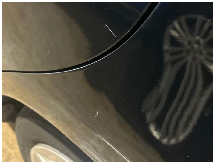
12: Door nsr Scratched UpTo 25mm Thru Paint
