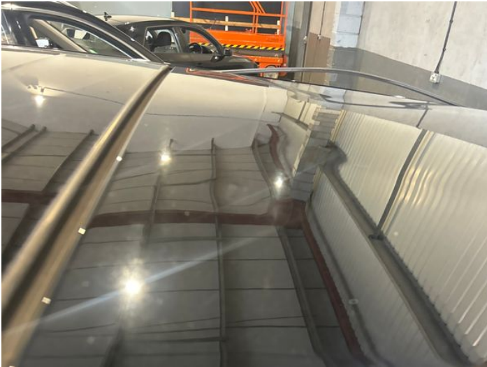
21: Roof Dented Over 30mm
