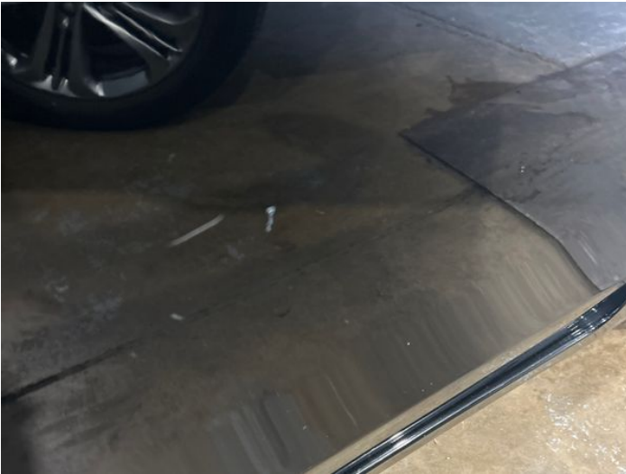
3: Door osf Scratched UpTo 25mm Thru Paint
