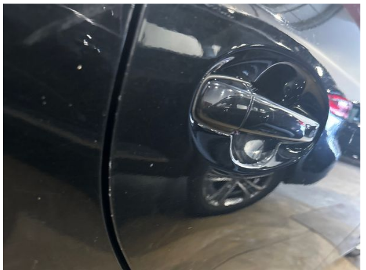
8: Door osr Chipped Edge Chip
