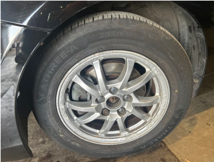
15: Wheel nsf Corroded Light
