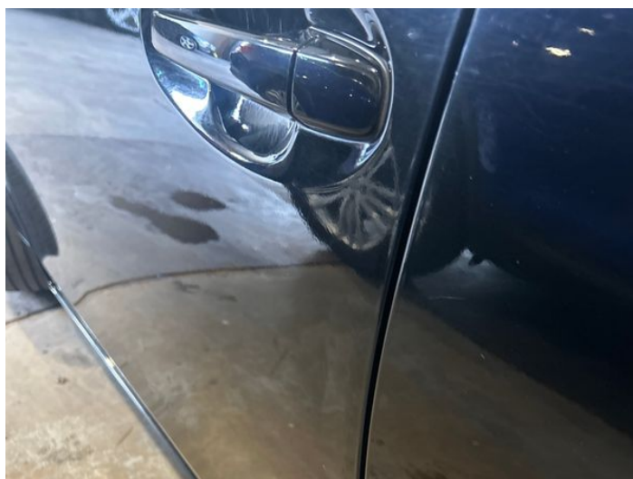
14: Door nsf Dented Over 30mm
