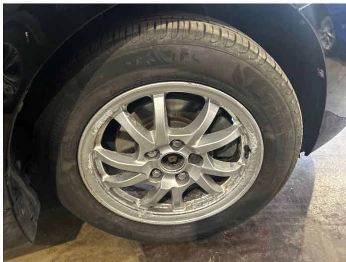
2: Wheel of Corroded Light
