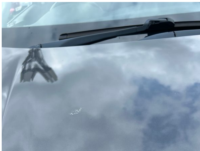
10: Bonnet Poor Previous Repair Paint Flake
