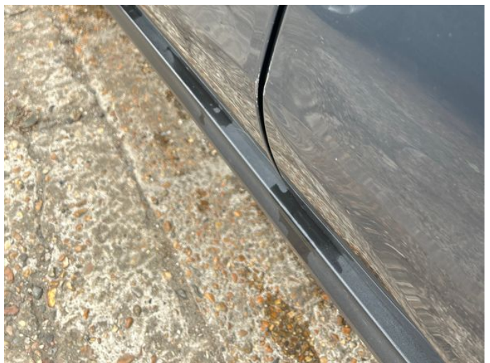
8: Door nsf Chipped Edge Chip
