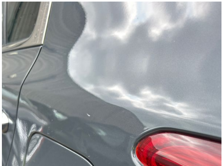
6: Qtr Panel nsr Dented Between 10mm + 30mm
