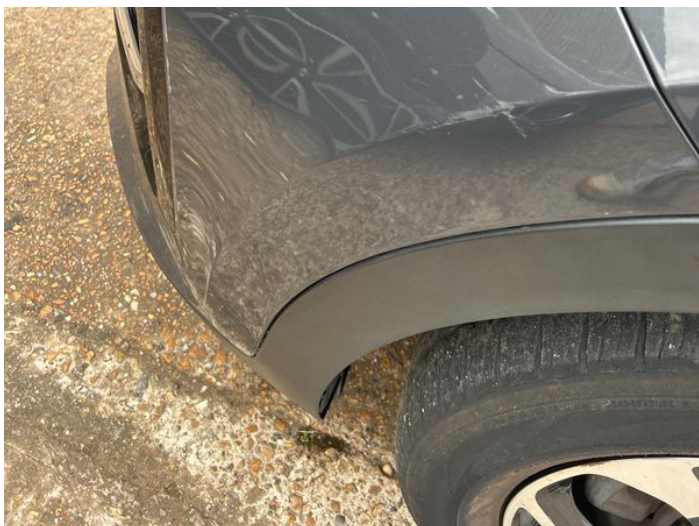
9: Bumper Front Scratched 25 to 100mm Thru Paint
