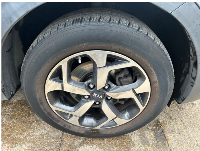
1: Wheel osf Corroded Light
