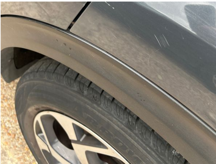
5: Qtr Panel nsr Scratched UpTo 25mm Thru Paint
