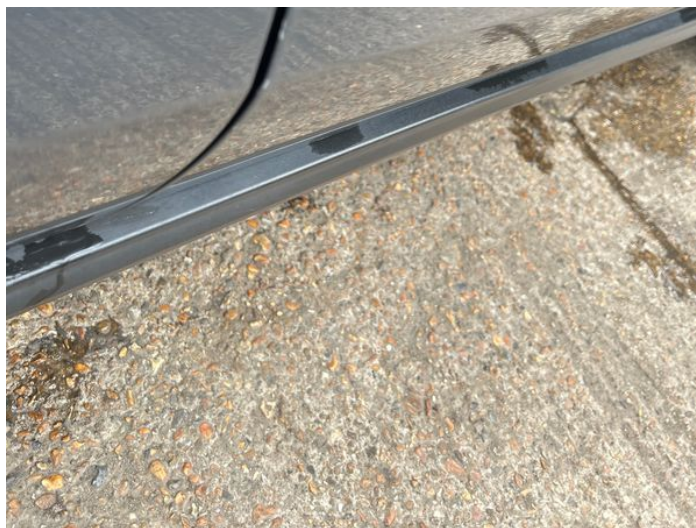
2: Door osf Chipped Edge Chip
