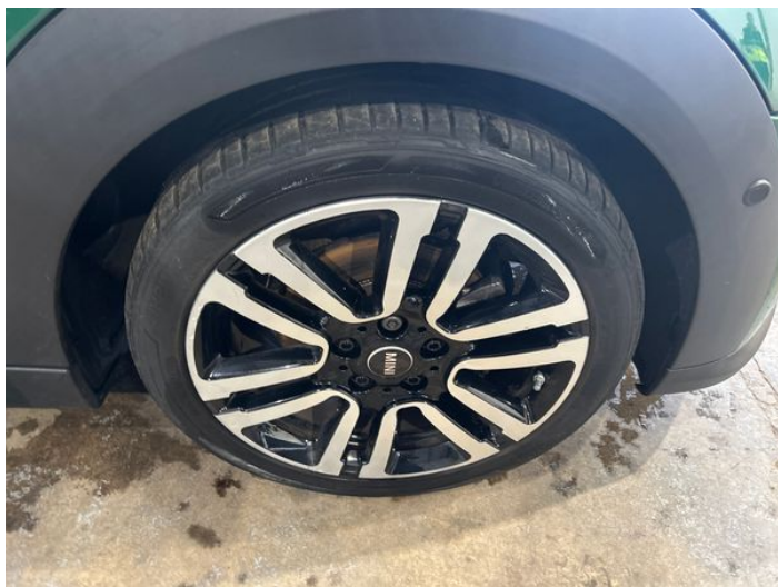
1: Wheel osf Corroded Light
