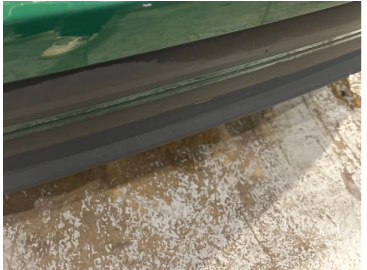
4: Bumper Rear Chipped 1 To 5
