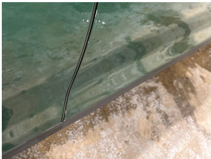
2: Door osf Chipped Edge Chip
