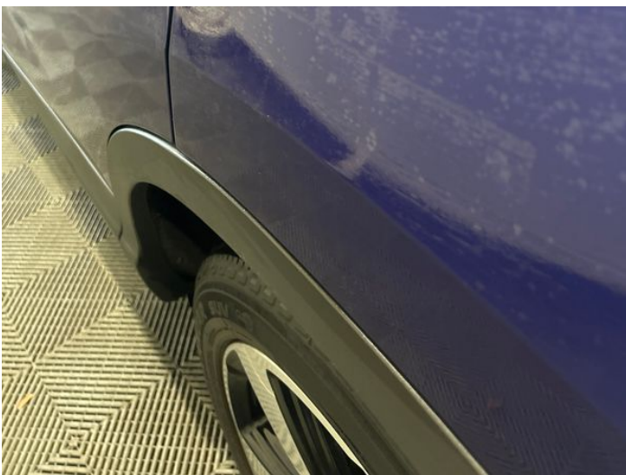
7: Qtr Panel nsr Dented Over 30mm
