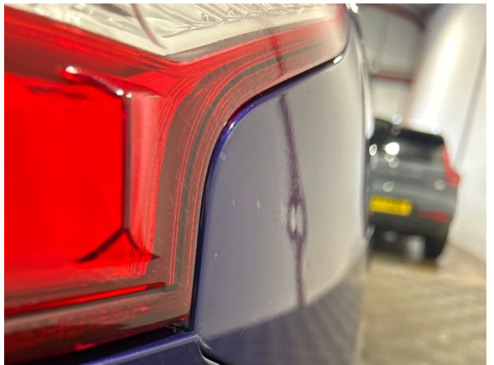
6: Qtr Panel osr Dented With Paint Damage
