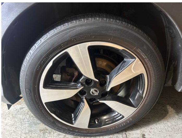
1: Wheel nsf Scratched Over 50mm
