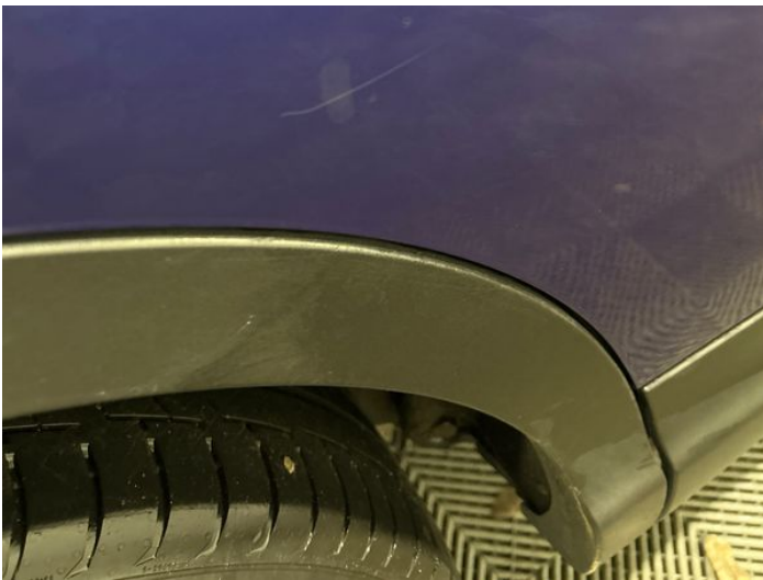
5: Door osr Scratched Over 25mm Thru Paint
