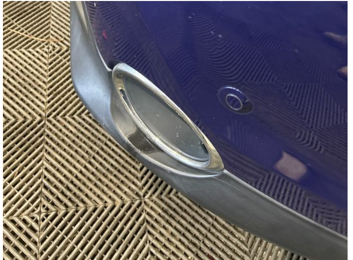
10: Bumper Front Chipped Multiple Chips
