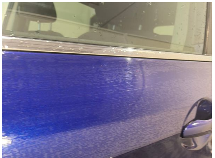
14: Door nsf Dented Between 10mm + 30mm
