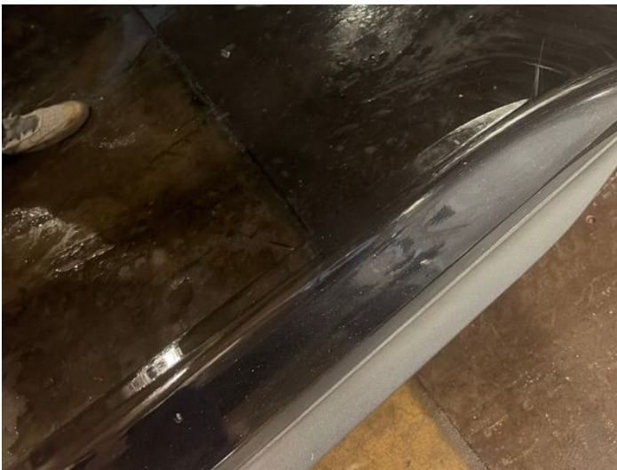
5: Door osf Scratched UpTo 25mm Thru Paint
