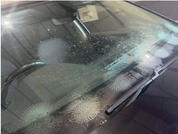
16: Screen Front Cracked Replace
