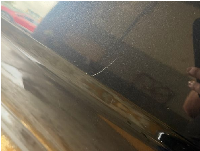
11: Door nsr Scratched Up To 25mm Thru Paint
