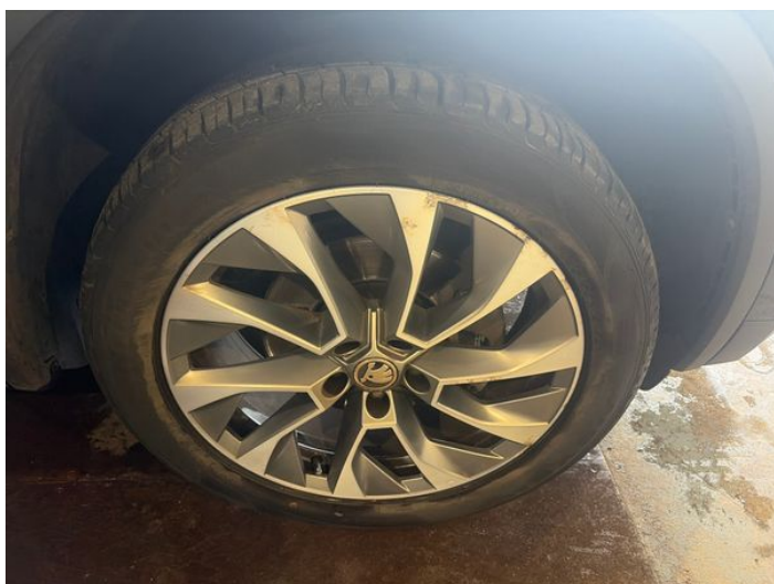
1: Wheel osf Corroded Light
