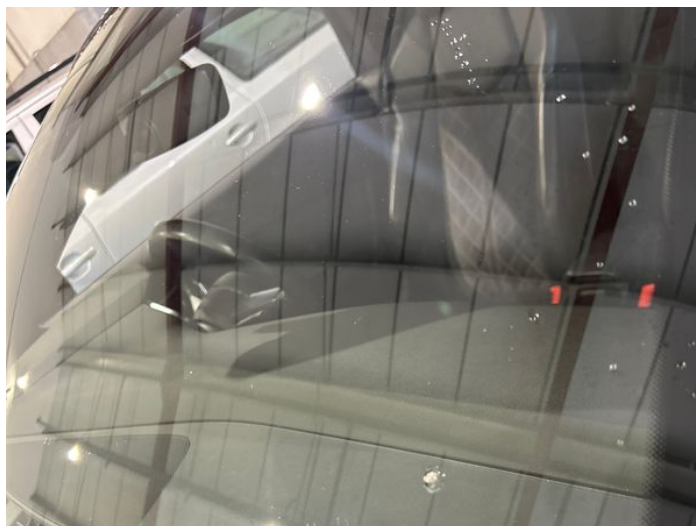
4: Screen Front Chipped UpTo 10mm
