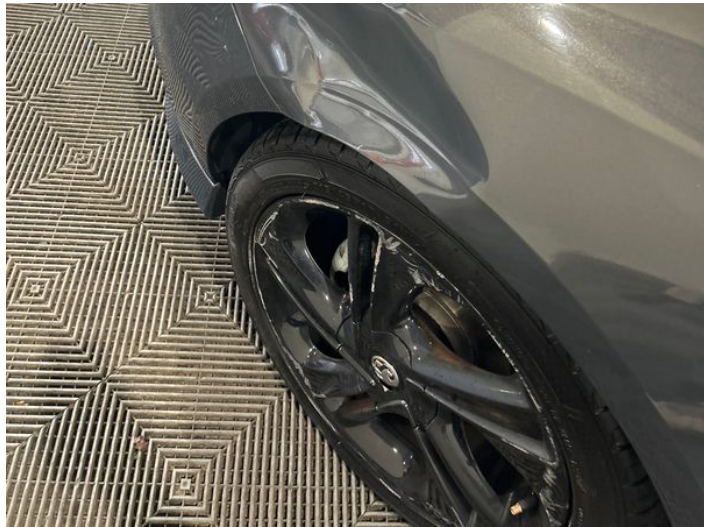
12: Wing nsf Dented Over 30mm
