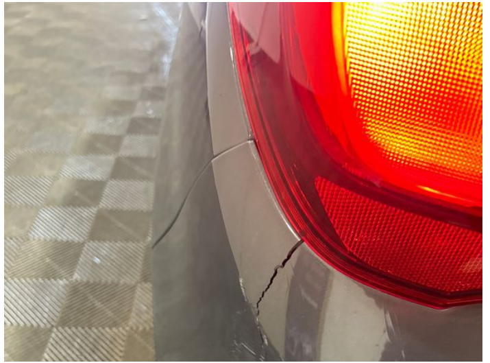
6: Bumper Rear Cracked Over 25mm
