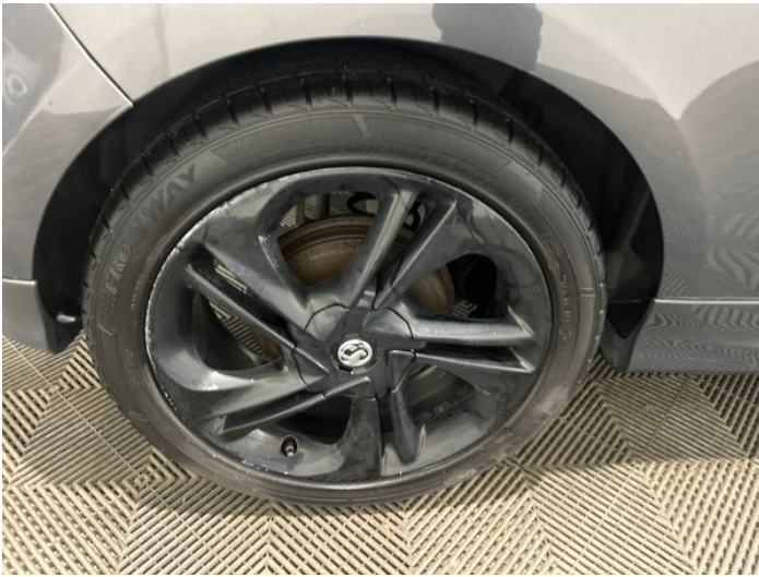
5: Wheel osr Scratched Over 50mm
