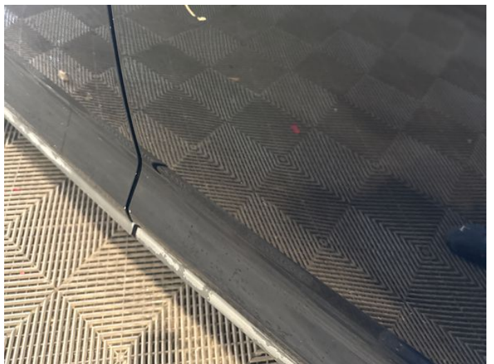
8: Door nsr Dented Between 10mm + 30mm
