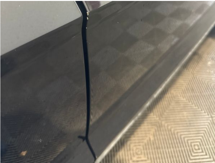
17: Door osf Scratched UpTo 25mm Thru Paint
