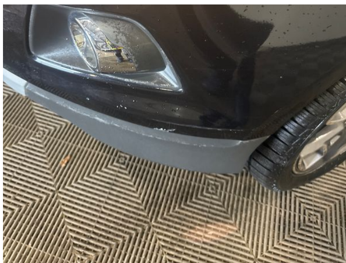
2: Bumper Front Scratched Over 100mm Thru Paint
