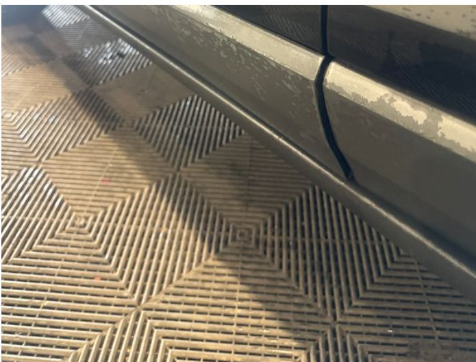
7: Door nsf Chipped 1 To 5
