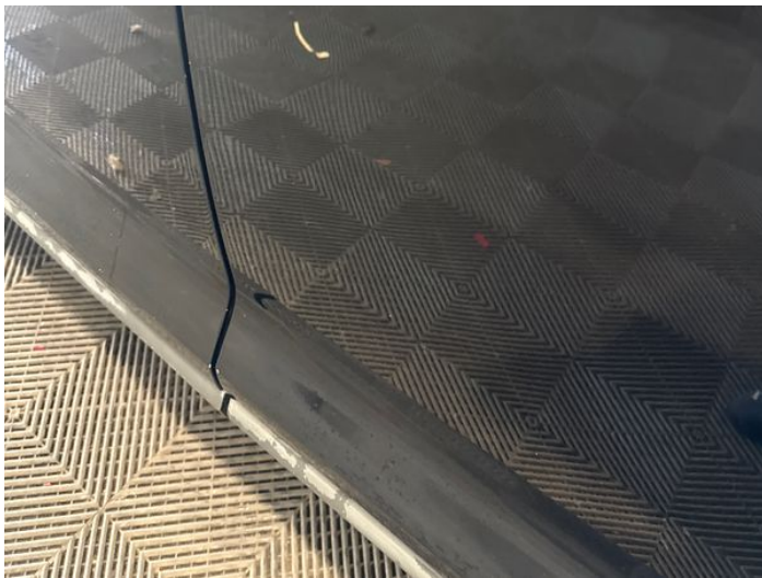
9: Door nsr Scratched UpTo 25mm Thru Paint
