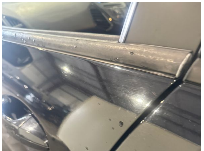
20: Door nsf Dented Between 10mm + 30mm
