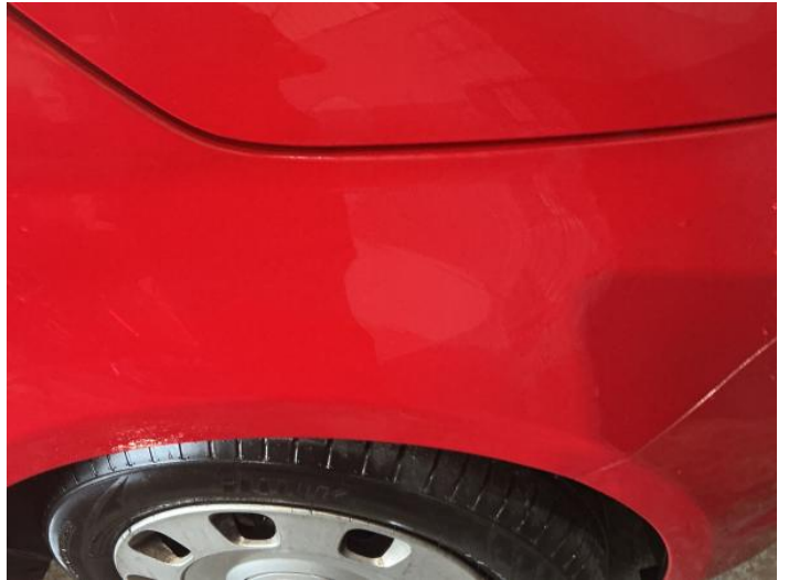
4: Wing osf Scratched UpTo 25mm Thru Paint
